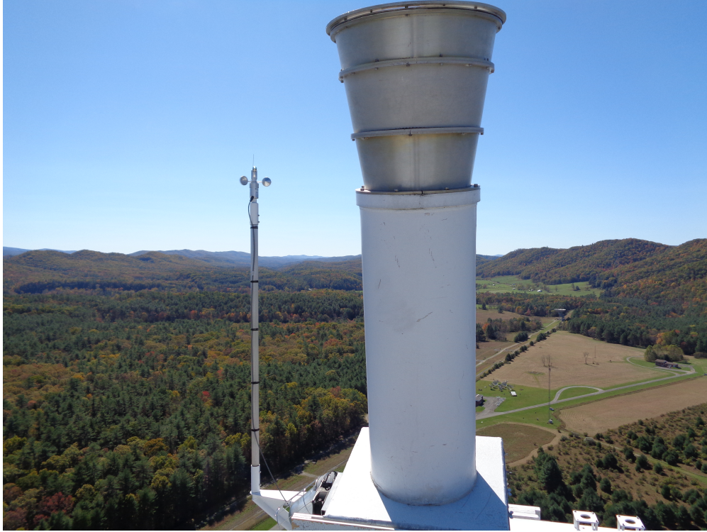
Figure 5: Anemometer for weather station #3, located above the subreflector and nearby to the current holography reference antenna, which is shown in the foreground (Credit: Bob Simon)
