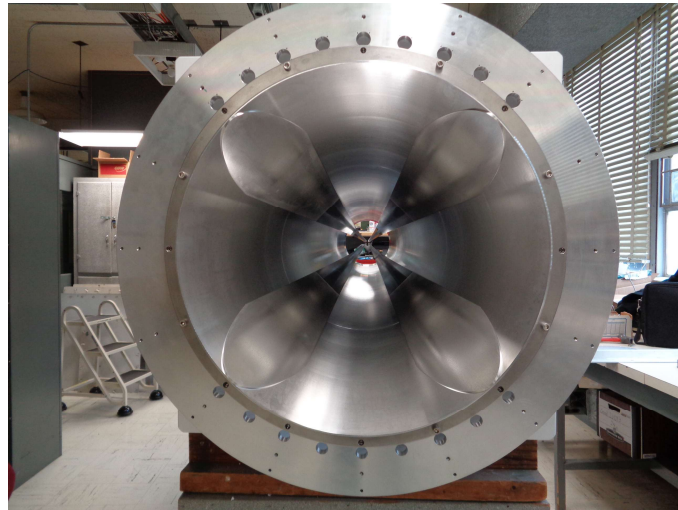
Figure 2. View of the aperture at ridge end where the thermal gap is located. The quartz spear, warm section of the feed outside the dewar, and corrugation sections are not installed. The total length is 1.839m with 1.2m inside the dewar. The aperture diameter is 0.9m extended to 1.590m with addition of the corrugated cone. The input circular WG diameter is 0.164m.
