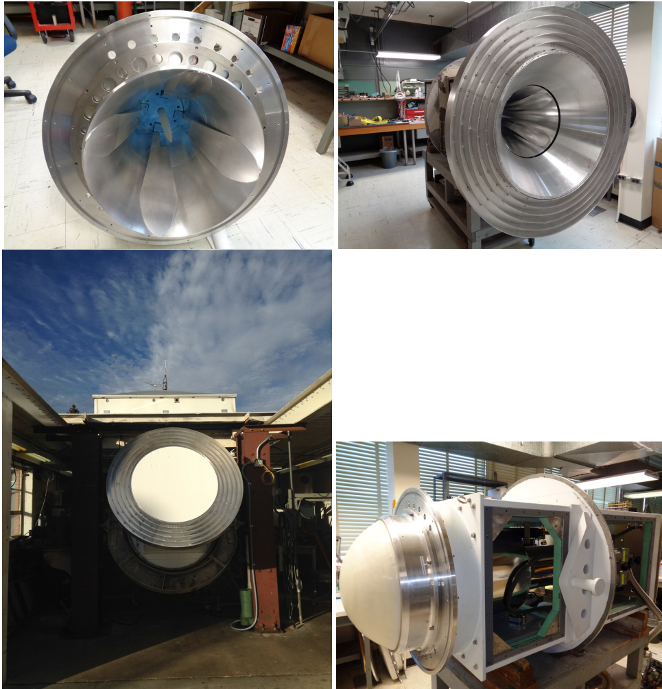
Figure 1: The UWBR feed in various states of assembly. Clockwise from upper left: The lower feedhorn with the ridges and dielectric spear; the assembled feedhorn and corrugations (the spear is not installed); the lower feedhorn with the vacuum window installed; the fully assembled receiver during testing in the Outdoor Test Facility.
