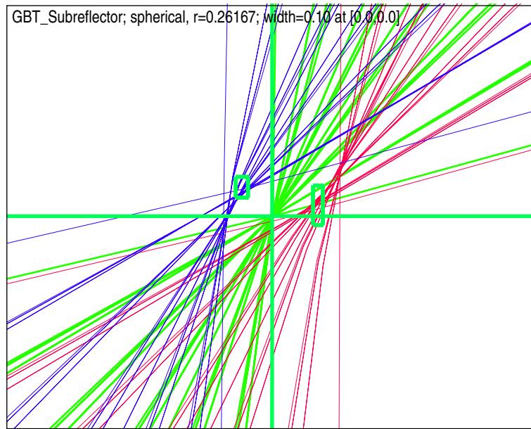
Figure 3: The three foci near the  $F_1$  focus (Prime focal plane)
