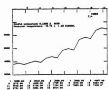
At the 12-meter telescope, the observing and analysis procedures are TPTIP for a total power tip or SPTIP for switched power data. A TPTIP example is shown to the right.
