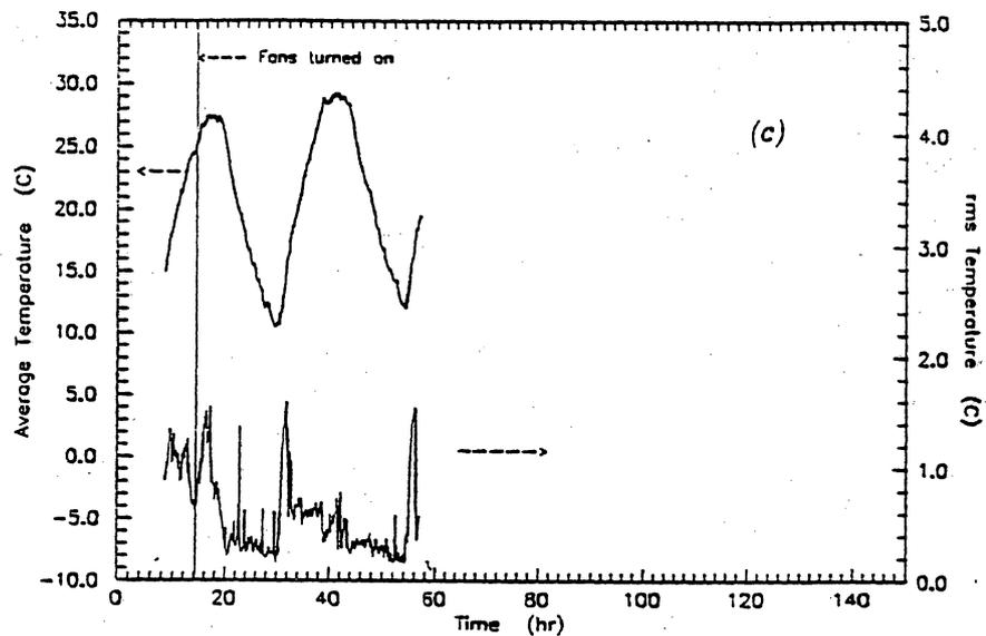
Figure 3. Average temperature in the backing structure, and rms variation of sensor readings from the mean.
