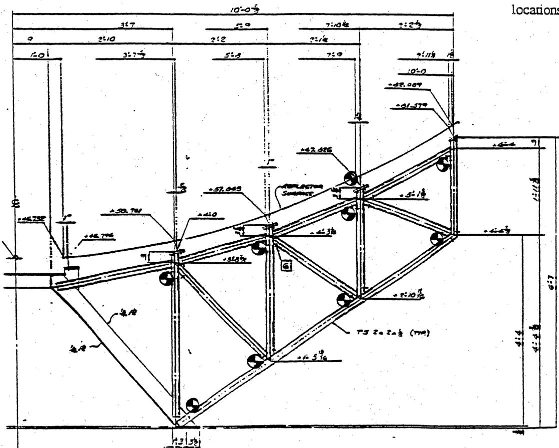
Figure 1. Drawing of backing structure truss showing location of thermistors.
