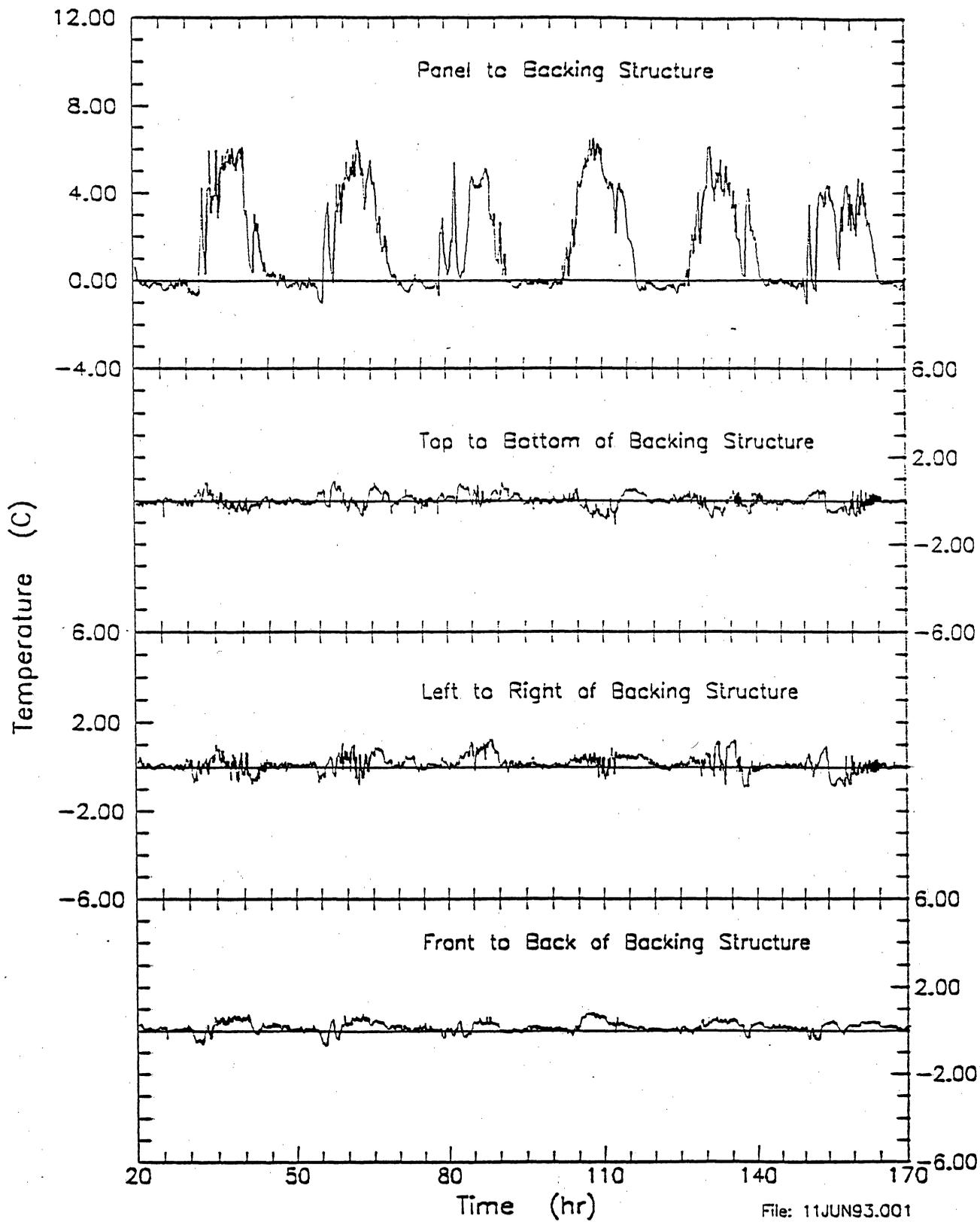
Figure 4. Differences between parts of the BS for 11<sup>th</sup> June 1993 data, fans and sunshades on.
