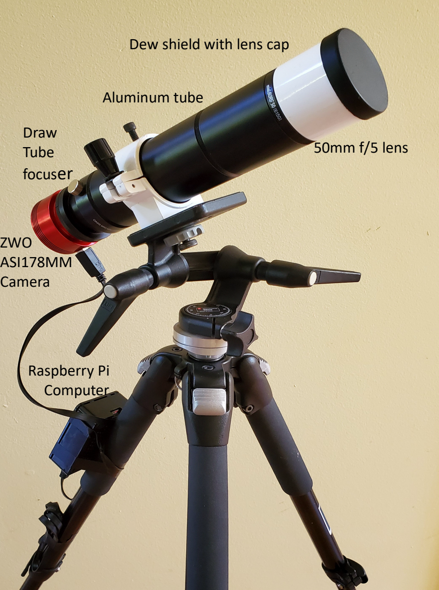
Figure 5.1: Prototype Optical Pointing system mounted on a tripod.
