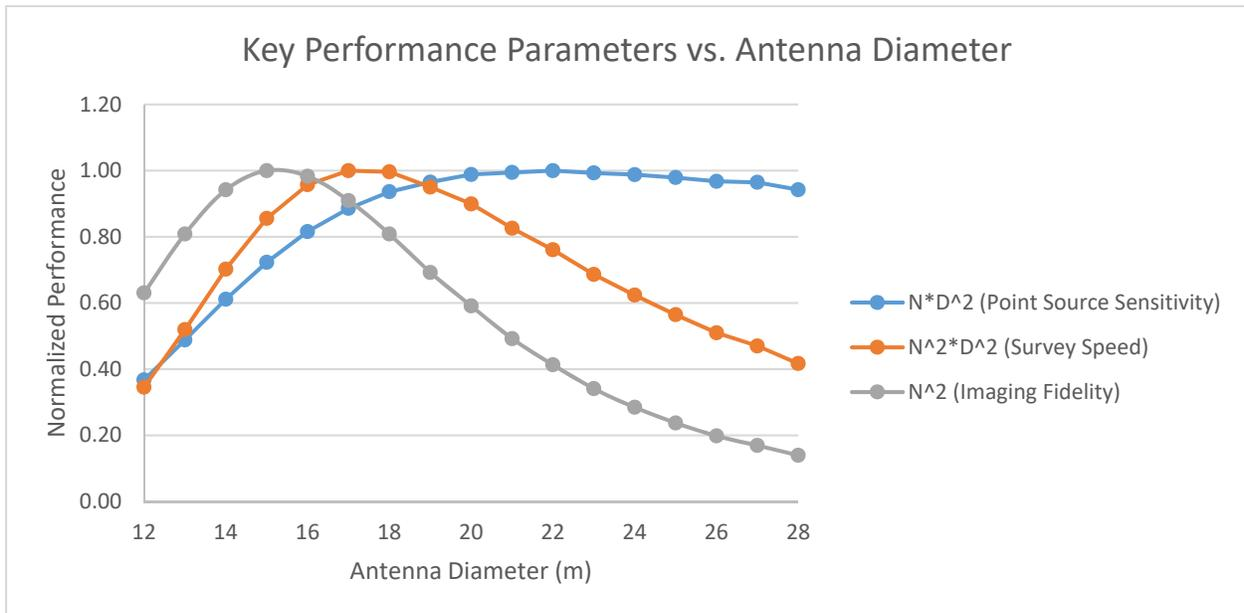
Figure 1 – Normalized KPP performance at fixed construction cost.
