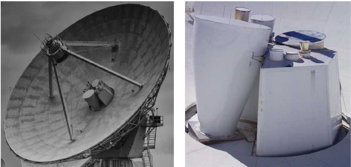
Figure 4 - Left: VLA antenna. Focus/rotation mechanism (FRM) is in the apex ring. Right: Close-in view of the feed cone. The large feeds are recessed well into the vertex cabin, to reduce blockage loss. The trade-off is a minor degradation in the phase efficiency and spillover at the low frequencies.
