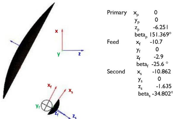
Figure 1. GRASP model of the ngVLA antenna.
