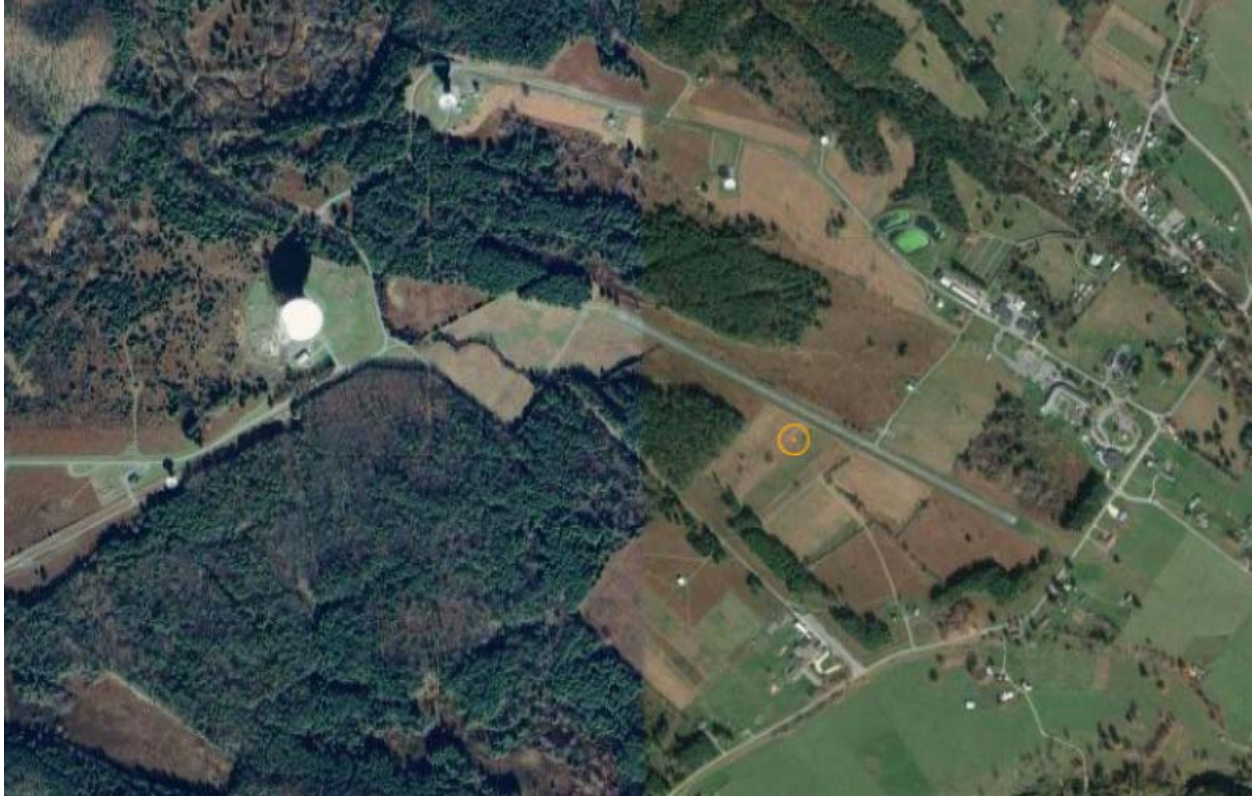
Figure 1 - Approximate site of the preferred ngVLA Site (in orange) near the middle of the air strip (the potato patch). [5] The site is approximately 1.2km from the GBT and 500m from the CHIME outrigger site. The main utility corridor (electrical and fiber service) is also approximately 500m to the north of this site.
