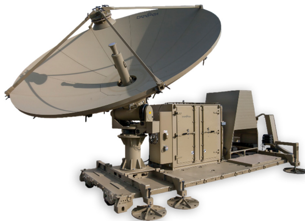
Figure 8 - Representative deployable Ku-band reference antenna package. DataPath DKET 3400 Series 4.0m system.
