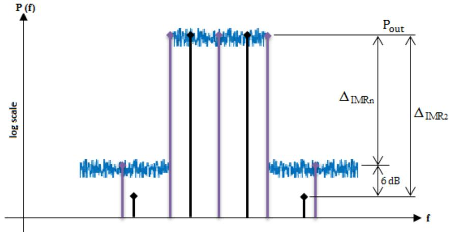
Fig. 6 Third-order intermodulation products for two-tone (**black**), three-tone (**purple** - for picture clarity, not all of 3<sup>rd</sup> order intermodulation products are shown), and the noise (**blue**) excitations of a weakly nonlinear RF system.
