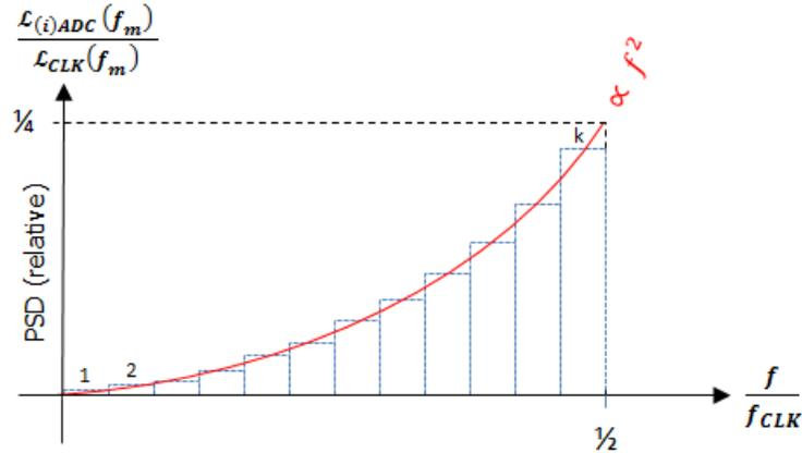
Fig. 5 Phase noise density transfer ratios for each of RFI tones across the 1<sup>st</sup> Nyquist band – ratios of single-sideband (SSB) phase noise spectral densities (relative to carrier) at the output of ADC v/s SSB phase noise spectral density of the sampling clock.
