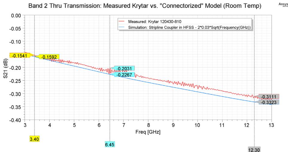
Figure 21. Thru Path Comparison of “Connectorized” Model to Measured Krytar 120430-810 at Room Temperature
