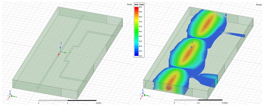
Figure 16. YBCO / MgO Band 2 Directional Coupler HFSS Model and E-field plot
