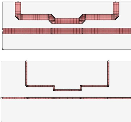
Figure 17. Sonnet subsections for Band 2 coupler simulations. Top) Conventional and Bottom) HTS
