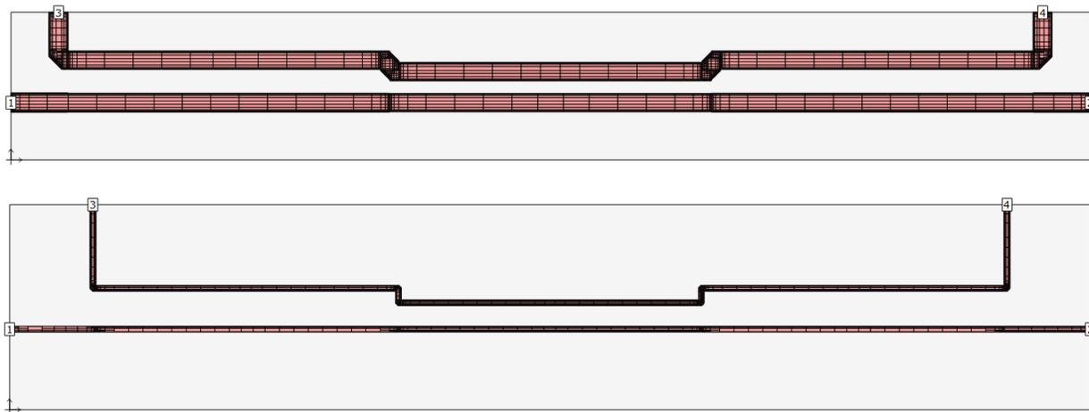
Figure 11. Sonnet subsections for Band 1 coupler simulations. Top) Conventional and Bottom) HTS
