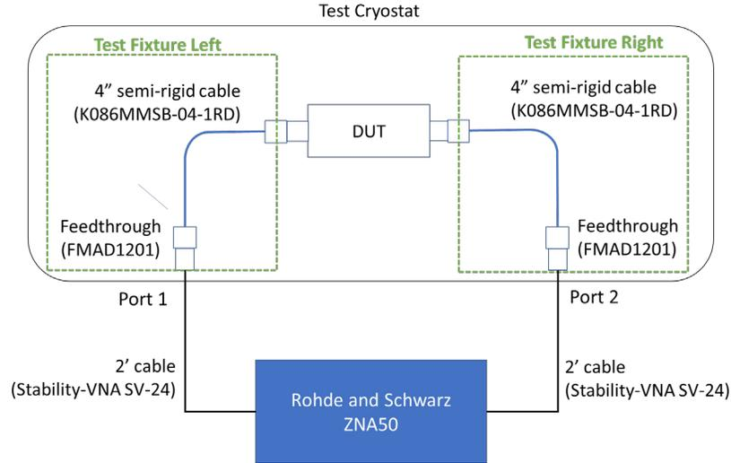
Figure 5. Test setup diagram of the Band 1 Krytar coupler (DUT) inside the test cryostat
