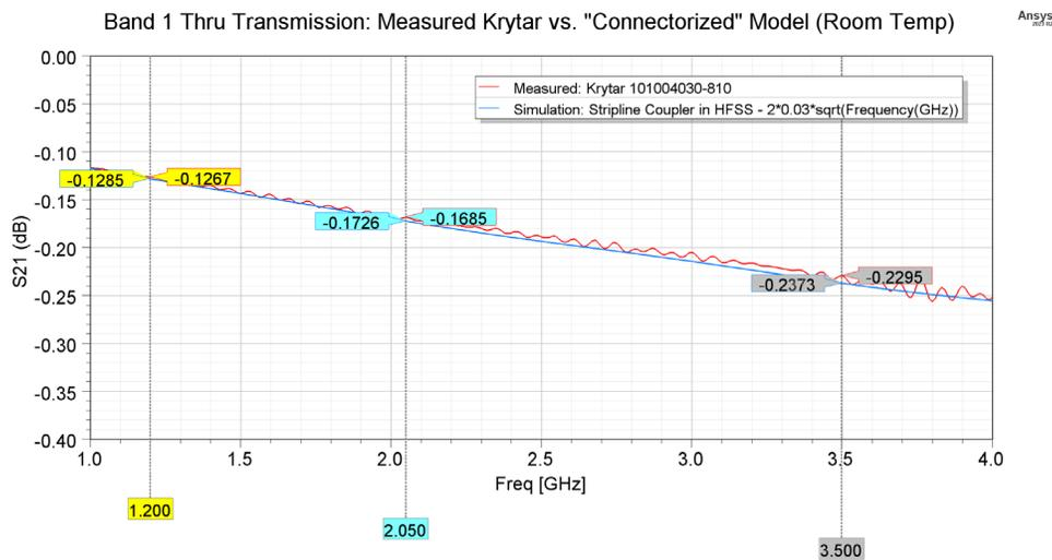
Figure 20. Thru Path Comparison of “Connectorized” Model to Measured Krytar 101004030-810 at Room Temperature
