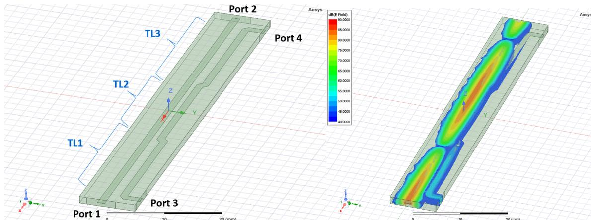
Figure 9. Copper / PTFE-composite Band 1 Directional Coupler HFSS Model and E-field plot
