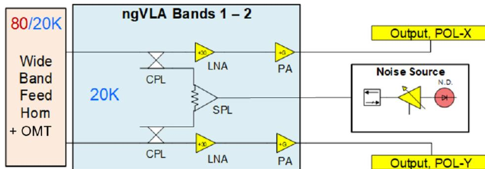
Figure 1. ngVLA Receiver front-end block diagrams [4]
