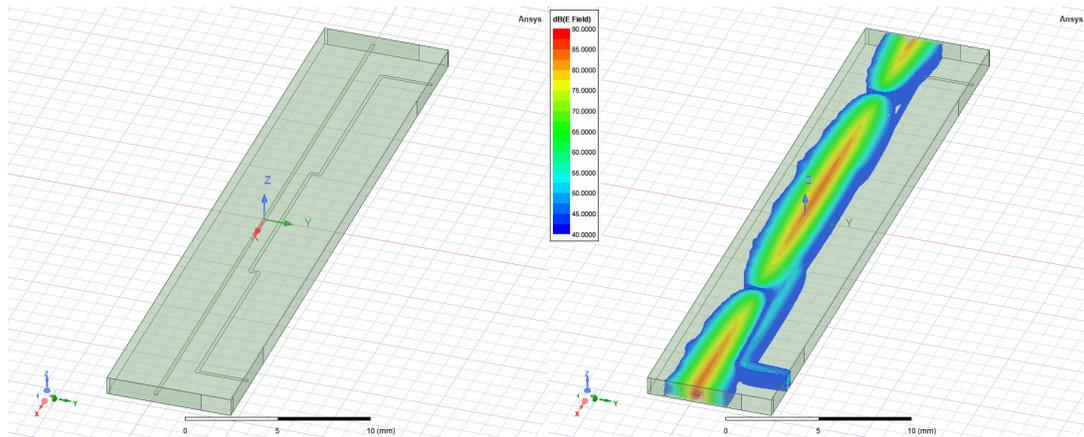
Figure 10. YBCO / MgO Band 1 Directional Coupler HFSS Model and E-field plot
