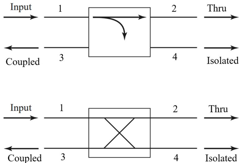
Figure 2. Two commonly used symbols for directional couplers, and power flow conventions [6]
