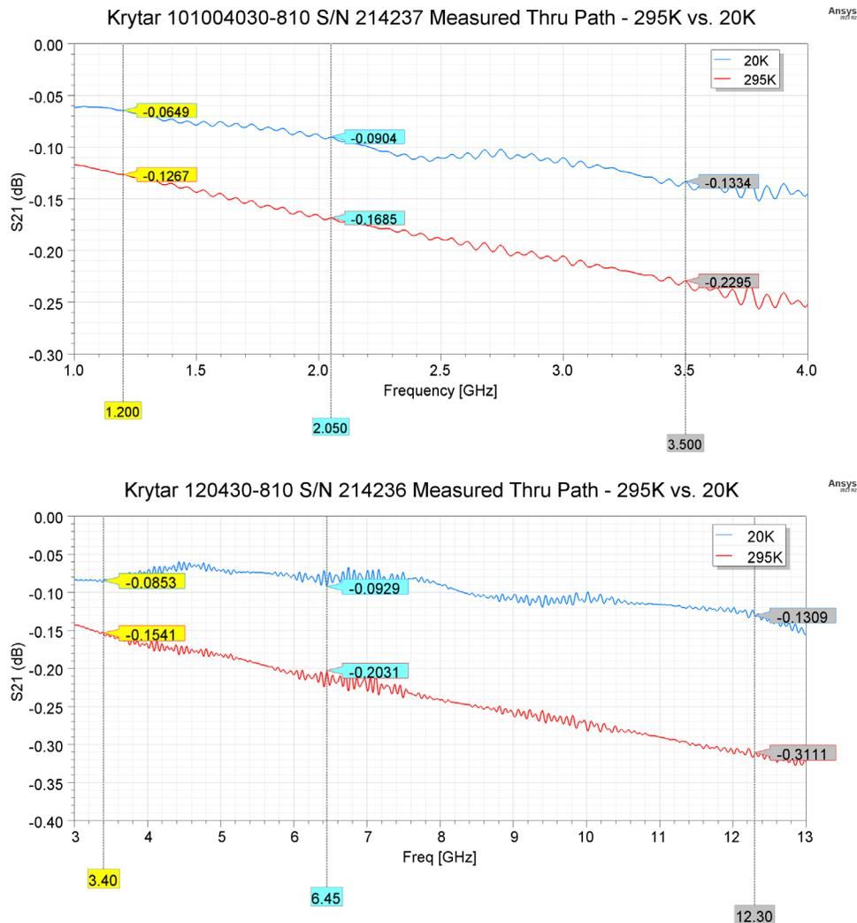
Figure 7. Measured transmissions of Band 1 and 2 Krytar couplers at 295 K (red trace) and 20 K (blue trace)
