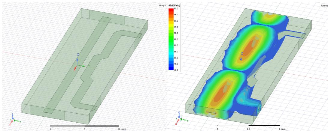
Figure 15. Copper / PTFE-composite Band 2 Directional Coupler HFSS Model and E-field plot
