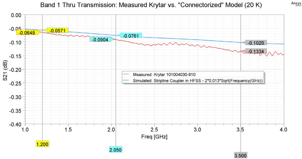
Figure 22. Thru Path Comparison of “Connectorized” Model to Measured Krytar 101004030-810 at 20 K
