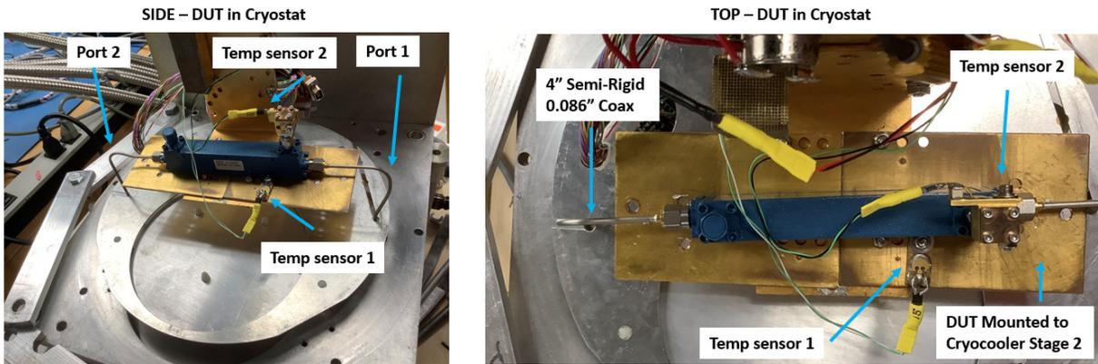
Figure 6. Band 1 Krytar coupler (DUT) mounted in test cryostat
