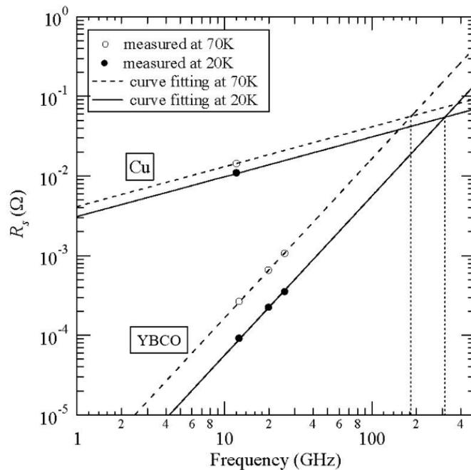
Figure 8. Measured YBCO surface resistance over frequency at 20K and 70K and curve fit lines [13]
