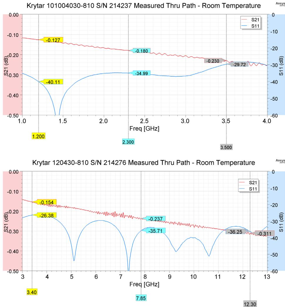
Figure 4. Krytar coupler thru path measurements at room temperature (295 K), for ngVLA Bands 1 (top) & 2 (bottom)
