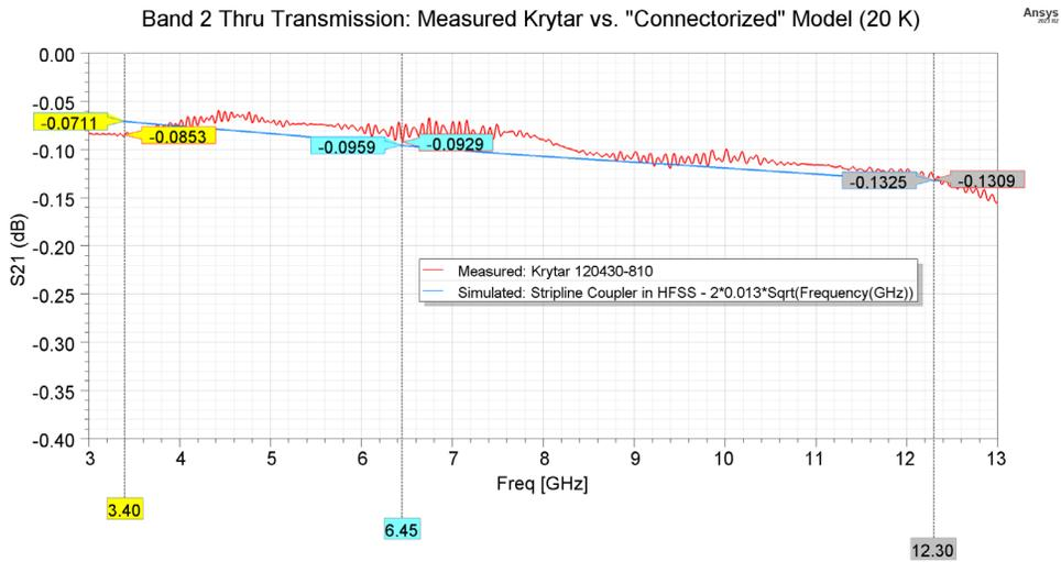
Figure 23. Thru Path Comparison of “Connectorized” Model to Measured Krytar 120430-810 at 20 K
