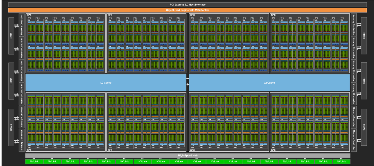
Figure 4: The internal structure of an NVIDIA H100 GPU, shown with the maximum complement of 144 Streaming Multiprocessors (SMs). The PCIe v5.0 x16 interface is shown at the top, HBM interfaces at each side, and the NVLink interface at the bottom. The detailed structure of the SM is shown in detail in Figure 5.
