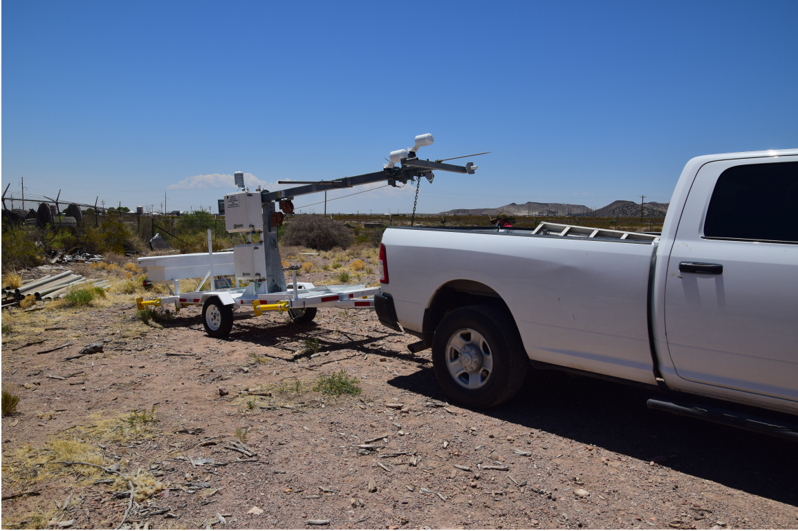
Figure 2: The Portable Weather Station being towed away from the EMRTC yard. Photo Credit: Justin Linford
