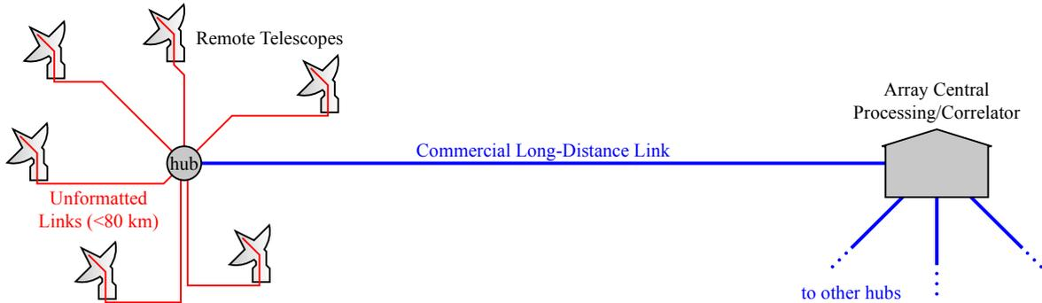
**Figure 4.** Illustration of two-stage data transmission, wherein the unformatted serial streams from a cluster of telescopes is gathered together and repackaged for delivery over longer distance through commercial data communications infrastructure.
