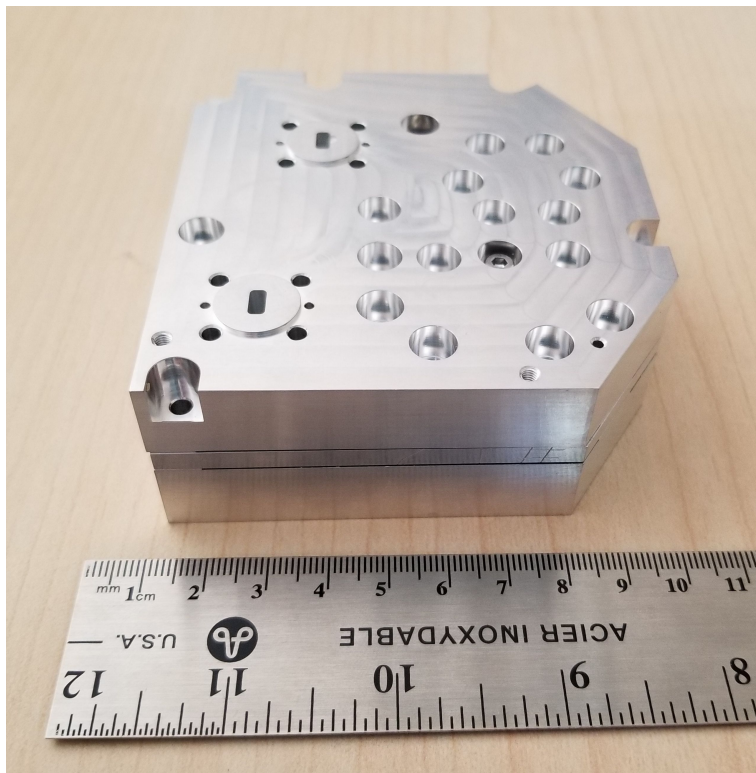
(b) Output face: 2 x WR 22 waveguide ports
