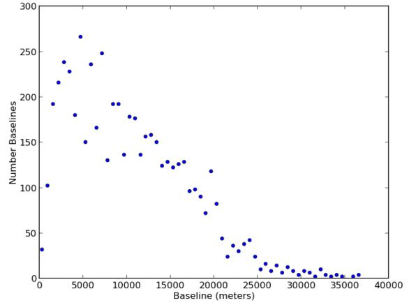
Figure 4: Left: Snapshot uv-coverage of the Spiral. Right: Histogram of baseline distribution.
