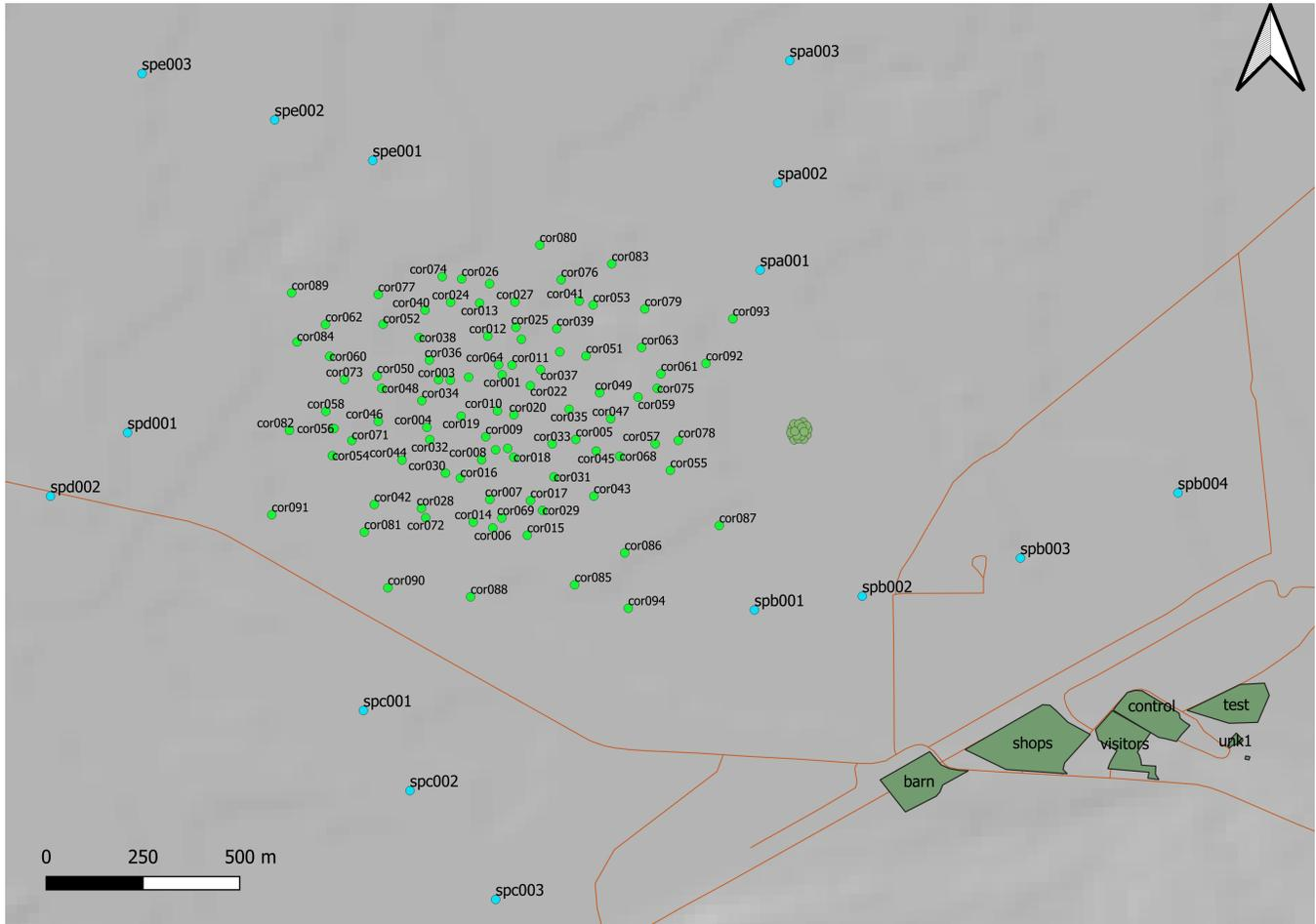
Figure 1: The Core configuration shown as light green circles. The inner spiral antennas are shown as cyan, to demonstrate the relationship. The SBA antennas are shown as darker green, about 700m east of the Core center. Also shown in this, and subsequent, figures is the terrain, and some of the roads and buildings.
