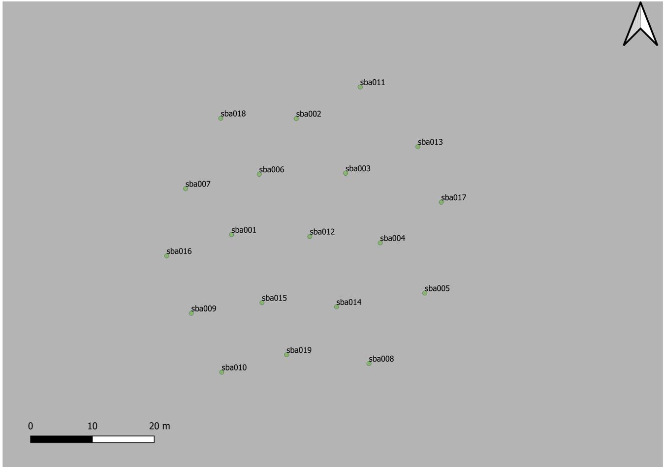
Figure 9: The Short Baseline array configuration shown as green circles.
