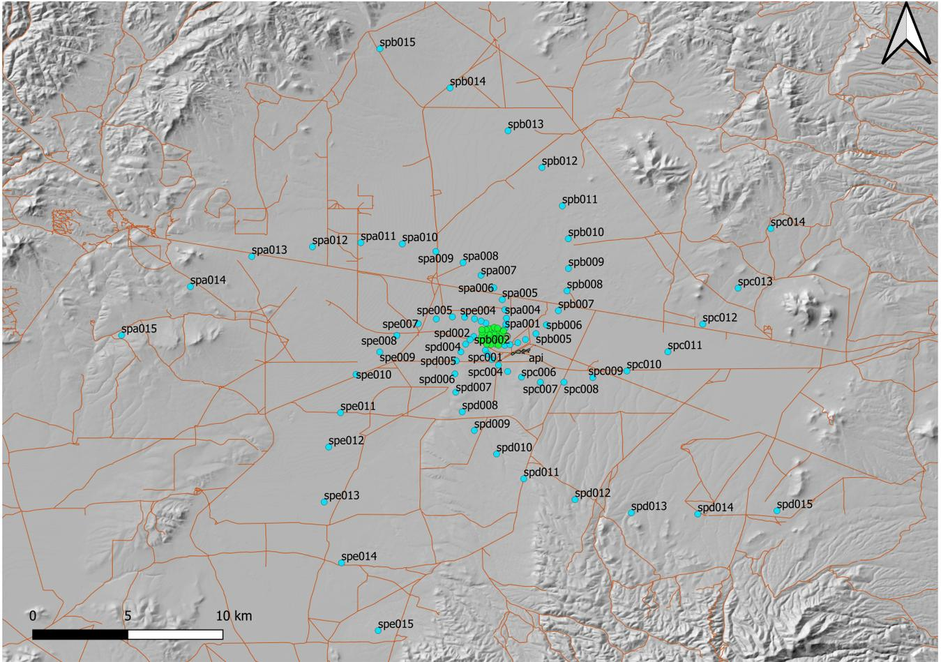
Figure 3: The Spiral configuration shown as cyan circles. The Core antennas are shown as green, to demonstrate the relationship.
