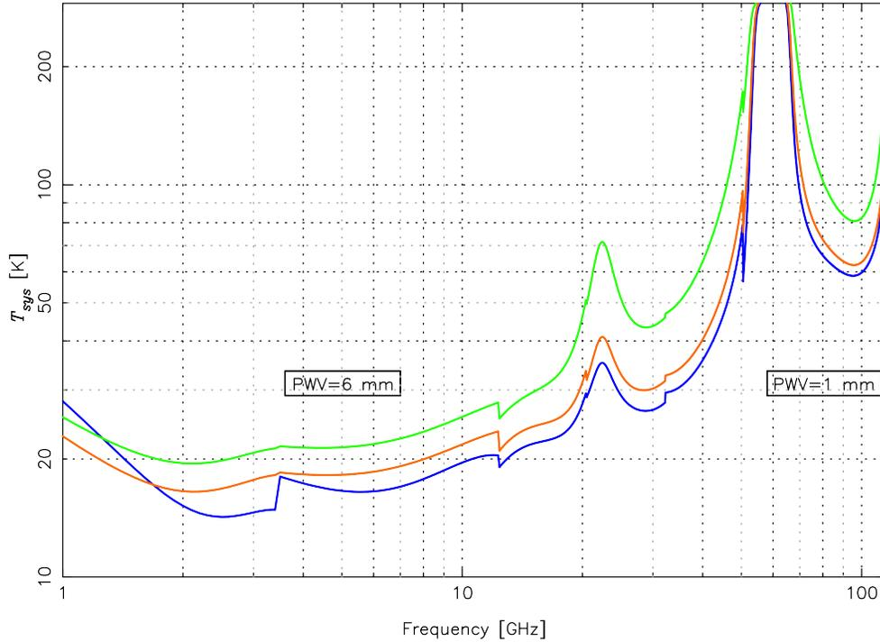
Figure 10. Calculation of  $T_{sys}$  vs. frequency, taking into account atmospheric emission, spillover, and receiver temperature. Color represents zenith angle: blue =  $0^\circ$ ; orange =  $45^\circ$ ; green =  $75^\circ$ .
