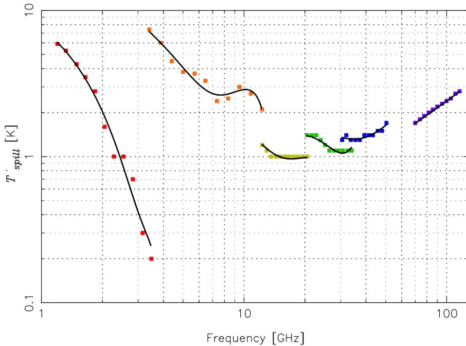
Figure 8. Values of  $T'_{spill}$  as a function of frequency. Calculated values are the colored dots (the six receiver bands for ngVLA are each a different color); the polynomial fits are the solid black lines.
