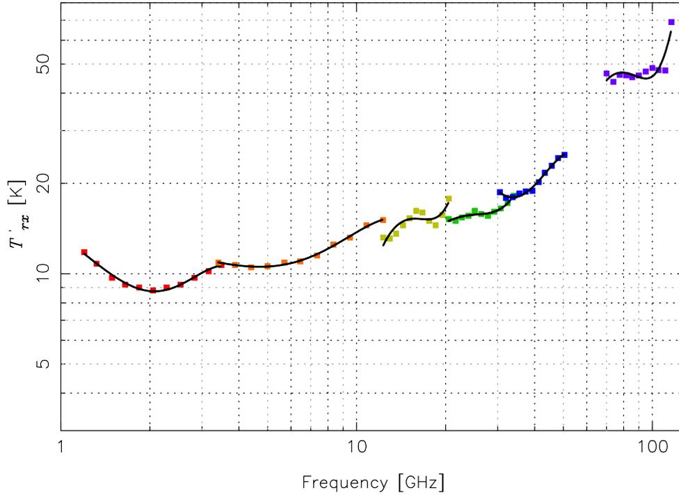
Figure 9. Values of  $T'_{rx}$  as a function of frequency. Calculated values are the colored dots (the six receiver bands for ngVLA are each a different color); the polynomial fits are the solid black lines.
