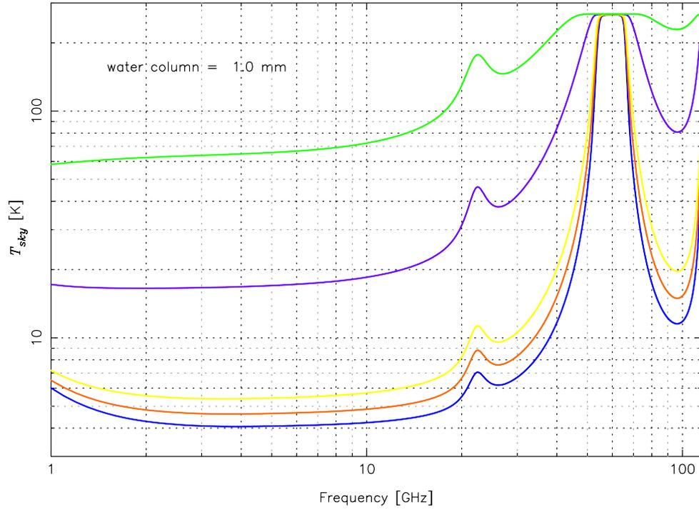
Figure 2. Contribution to the antenna noise temperature from the atmosphere ( $T_{sky}$ ) for  $PWV = 1$  mm. Colors are different zenith angles: blue =  $0^\circ$ ; orange =  $45^\circ$ ; yellow =  $60^\circ$ ; purple =  $85^\circ$ ; green =  $90^\circ$ .
