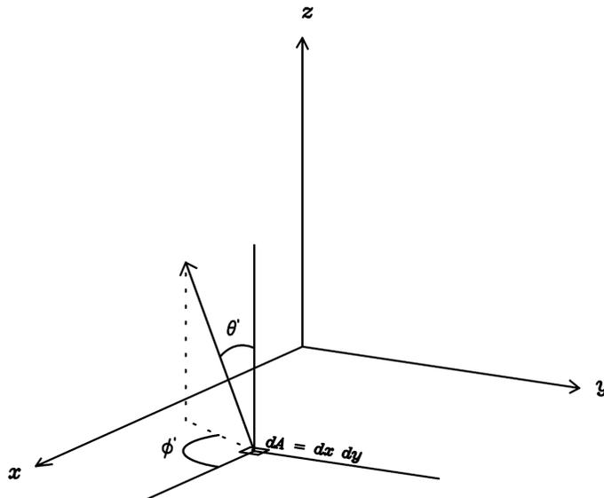
Figure 5. Geometry for direct ground emission contribution to  $T_{spill}$ .
