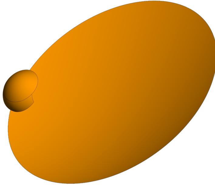
Figure 7. Model of main reflector, subreflector, and subreflector ground shield used for calculations of  $T_{spill}$ .
