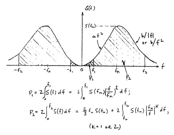
Fig. 1: Typical power spectrum of a locked oscillator, where f is the offset from the carrier frequency.  $P_1$  and  $P_2$  are the close-in and wideband noise powers considered in the text; they are derived by integrating the functions shown here.
