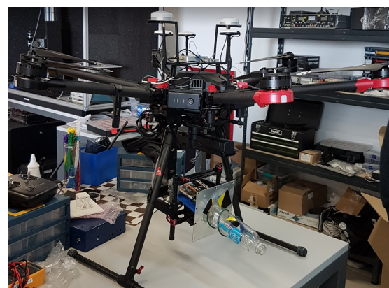
Figure 8: The hexacopter drone with a radio source payload tested at the Universidad Catolica of Santiago
