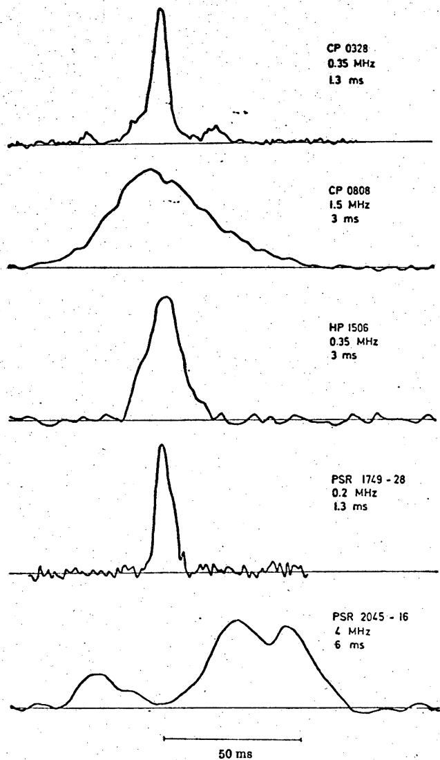
Fig. 5. Mean pulse profiles at 408 MHz over periods of 10 min on the five pulsars. For each source the bandwidth and overall resolution, including dispersion and time constant, are indicated. The aerial polarization was circular for the first three and linear for the other two.
