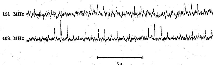
Fig. 3. A fast galvanometer recording of a train of pulses from CP 0328 received simultaneously at frequencies of 151 MHz and 408 MHz (on August 4). The dispersion delay of nearly six periods is evident.
