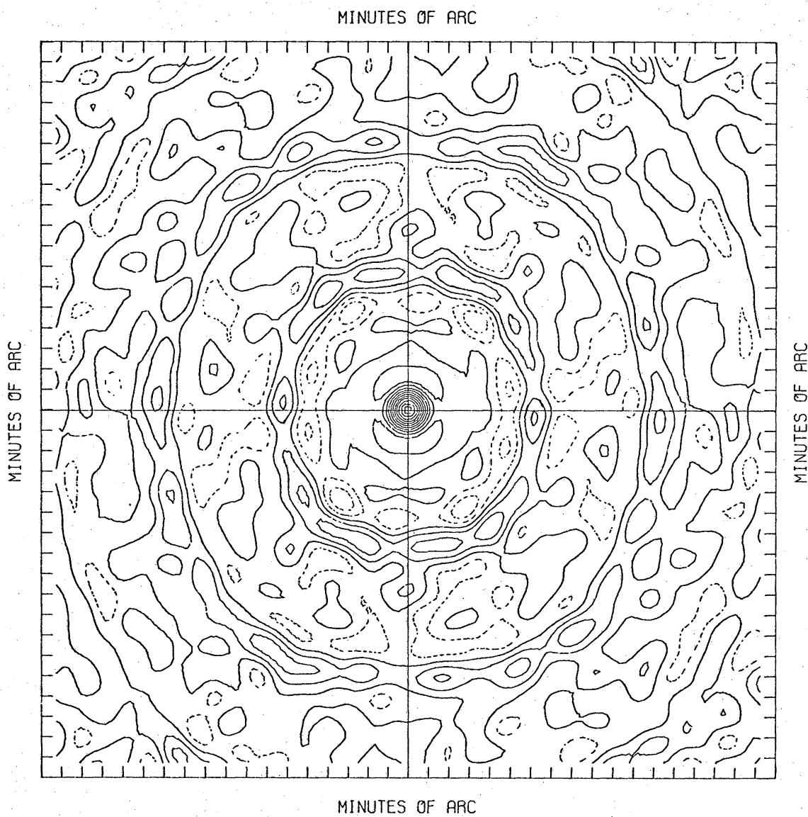
Figure 17a. 3C461, continuum frequency shift: dirty beam pattern, contour interval = 10%, large area.
