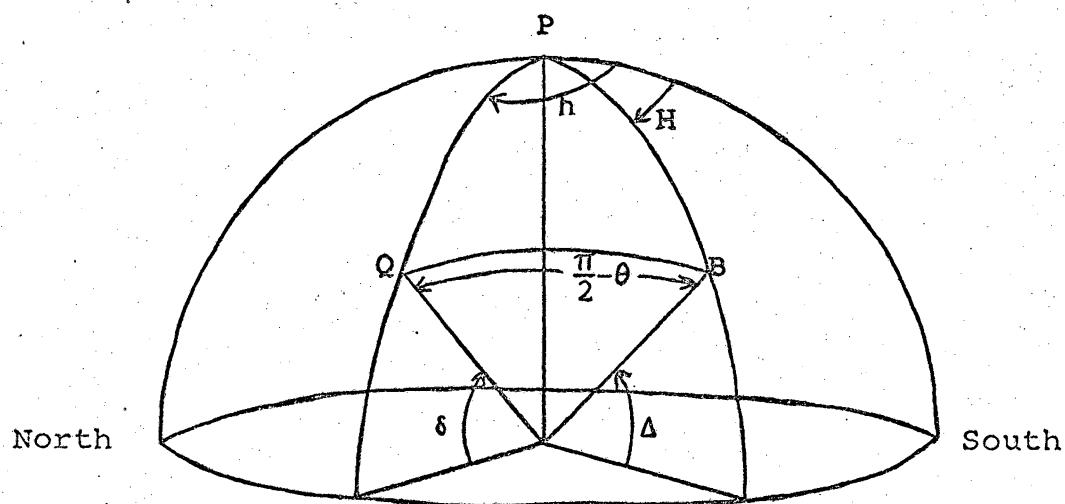
Figure A2. Celestial sphere with source (Q) and pole of baseline (B).
