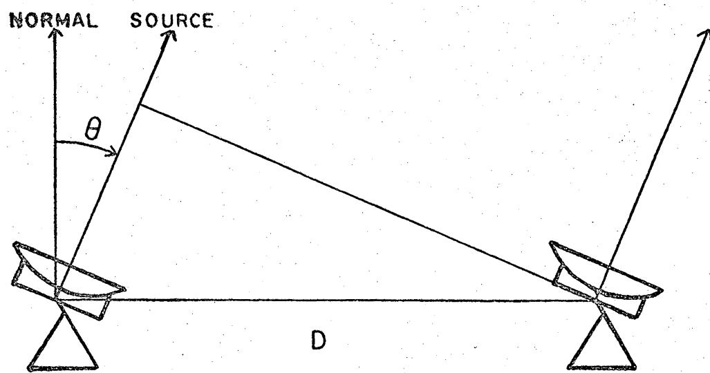
Figure A1. Geometry of two-element interferometer.
