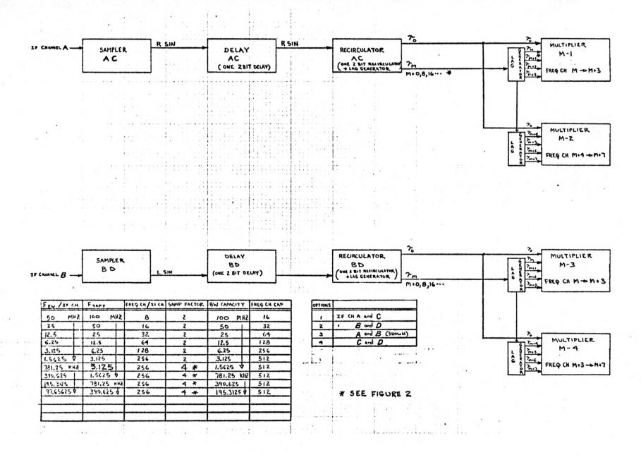
FIGUR E 4 FOUR BAND SPECTRAL LINE MODE
