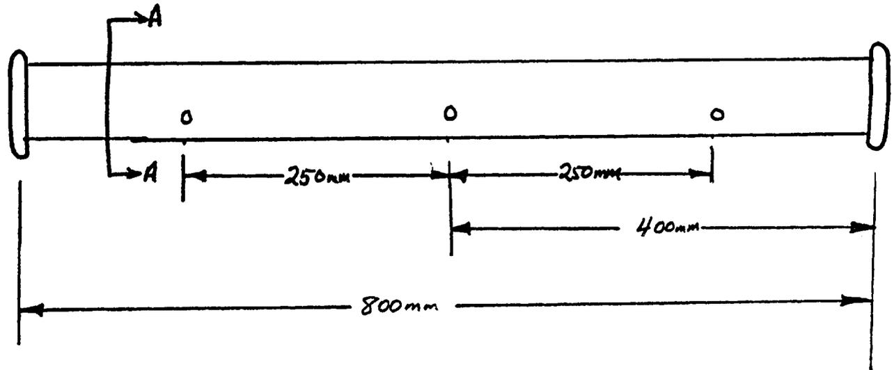
transducers are electronically summed, scaled and subtracted within the body of the mouse to provide an output of the deviation from straightness with a typical sensitivity of 14 V/millimeter. The radius of curvature is the inverse of the measured deviation  $\delta$ ,
