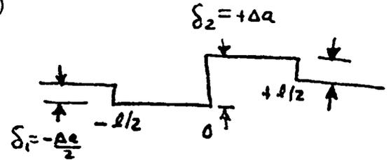
Response to an upward offset or diameter decrease ( $\Delta D = 2\Delta a$ ).
