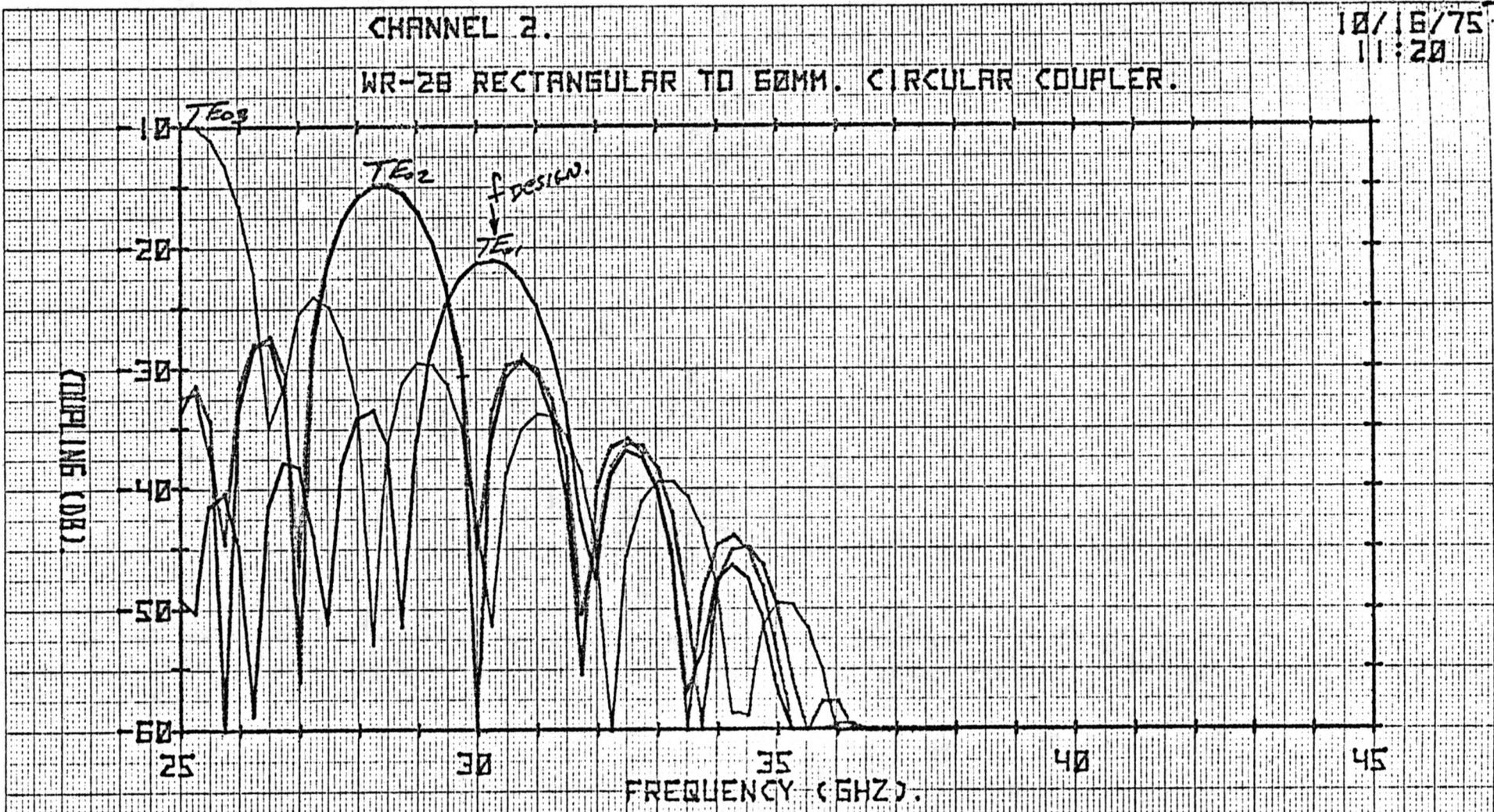
TE0 2 MODE, 32 COUPLING UNITS SPACED 2.530MM. APART.
