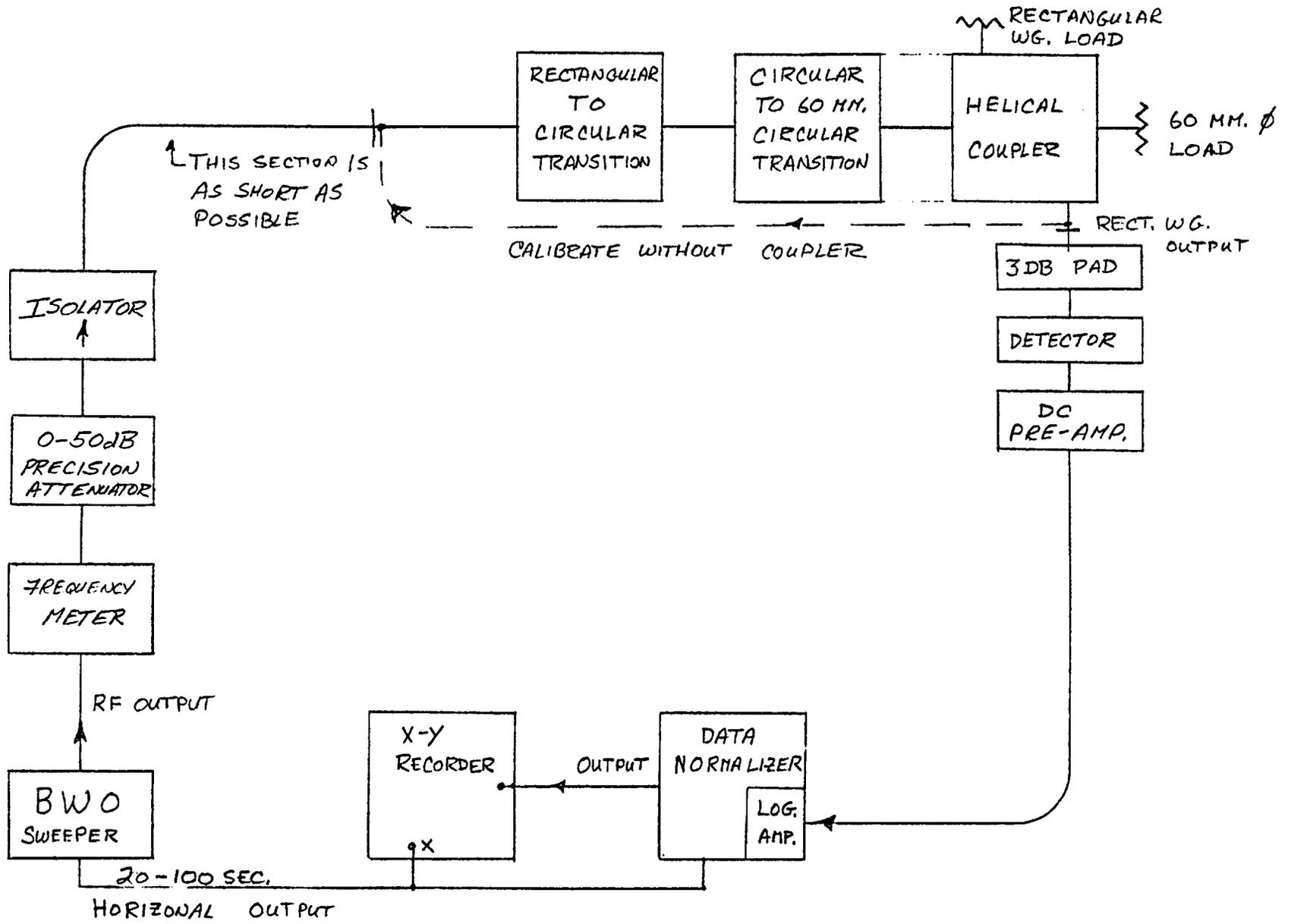
FIGURE 4.2a: MEASUREMENT OF TE<sub>01</sub> CIRCULAR TO TE<sub>10</sub> RECTANGULAR COUPLING
