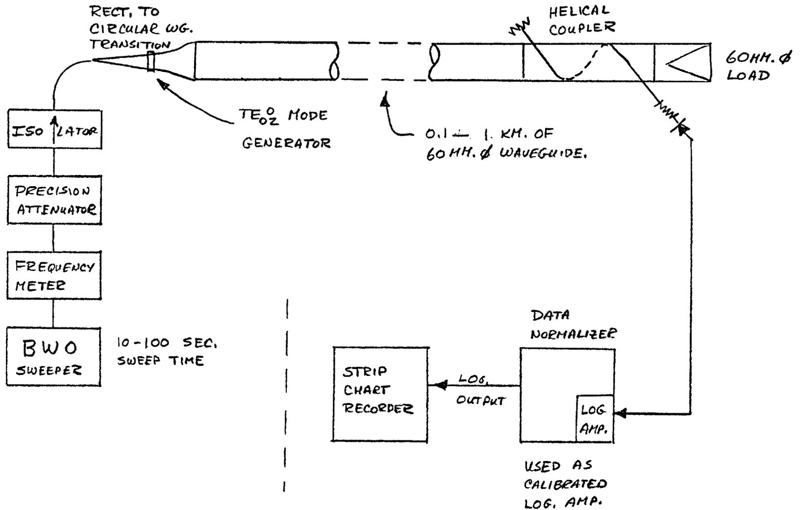
FIGURE 4.4: MEASUREMENT OF TE<sub>02</sub> CIRCULAR MODE DISCRIMINATION
