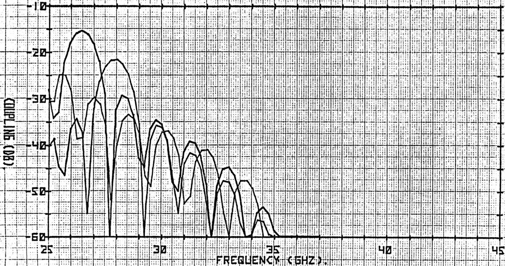
TE0 1 MODE, 78 COUPLING UNITS SPACED 2.750MM. APART.
