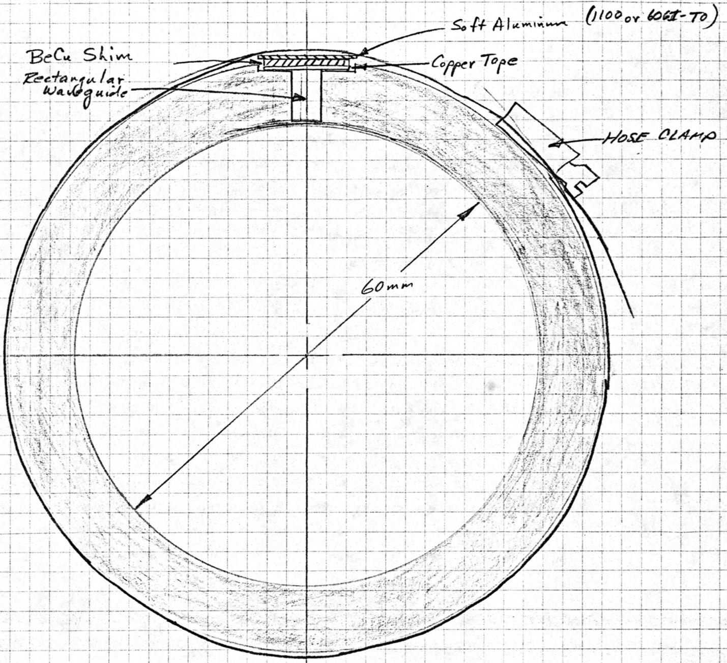
FIGURE 4.1: TEMPORARY SLOT COVER
