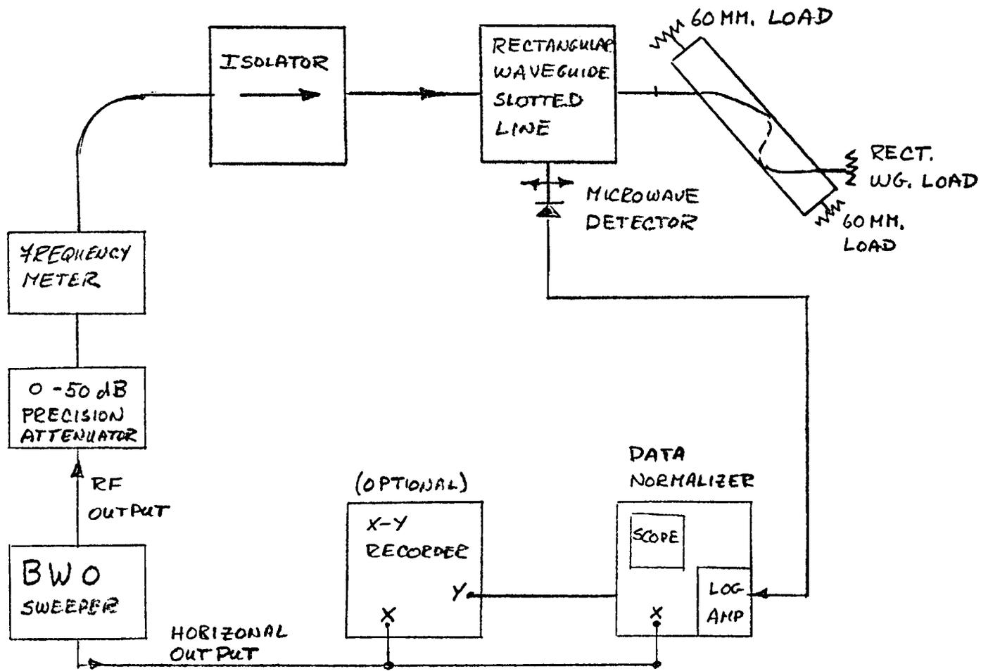
FIGURE 4.3: MEASUREMENT OF  $TE_{10}$  RECTANGULAR RETURN LOSS
