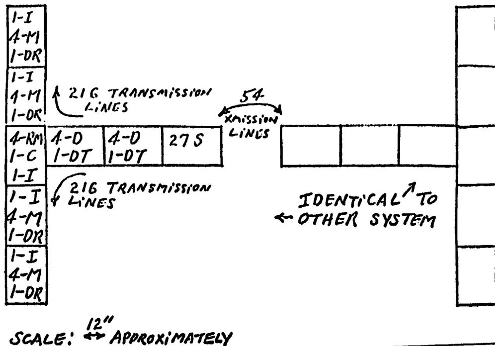
FIGURE III-5. VLA CONTINUUM AND SPECTRAL CORRELATOR, RACK ARRANGEMENT
