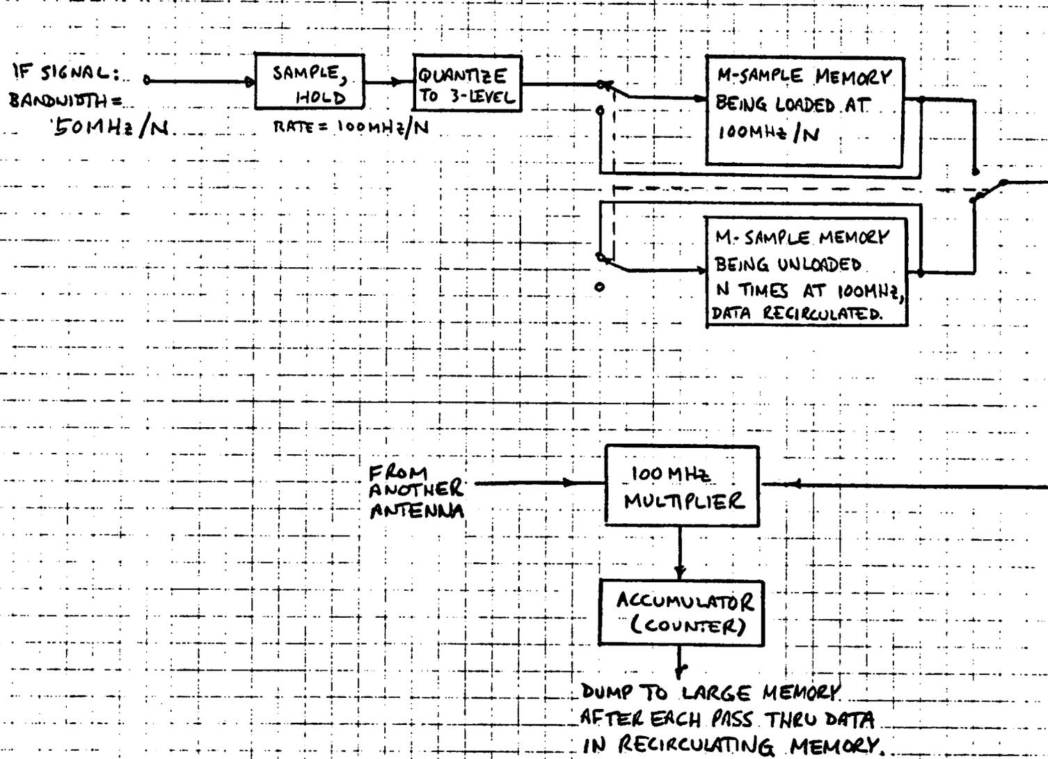
FIGURE III-2: THE RECIRCULATION CONCEPT
