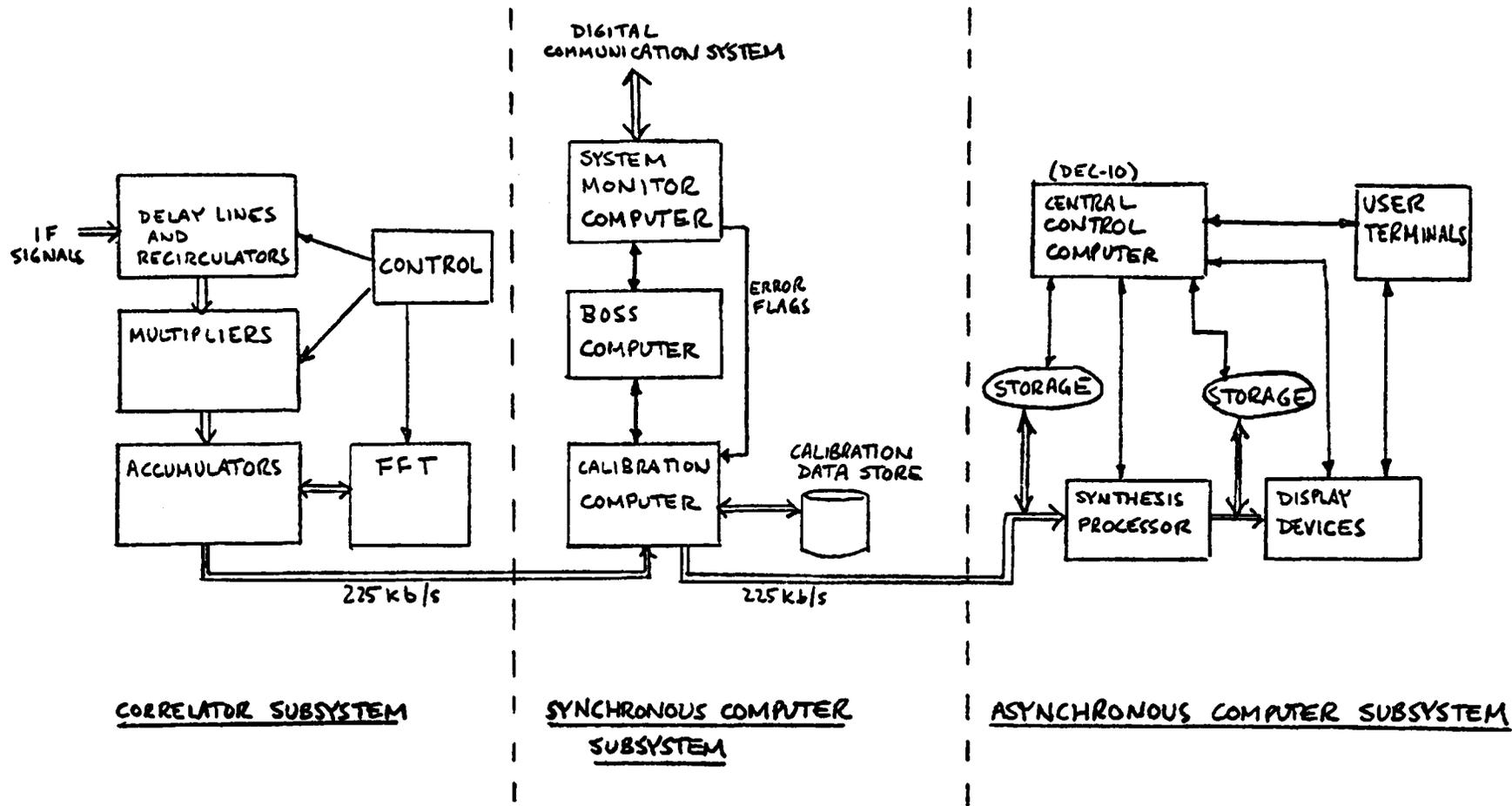
Figure III-1. System Block Diagram
