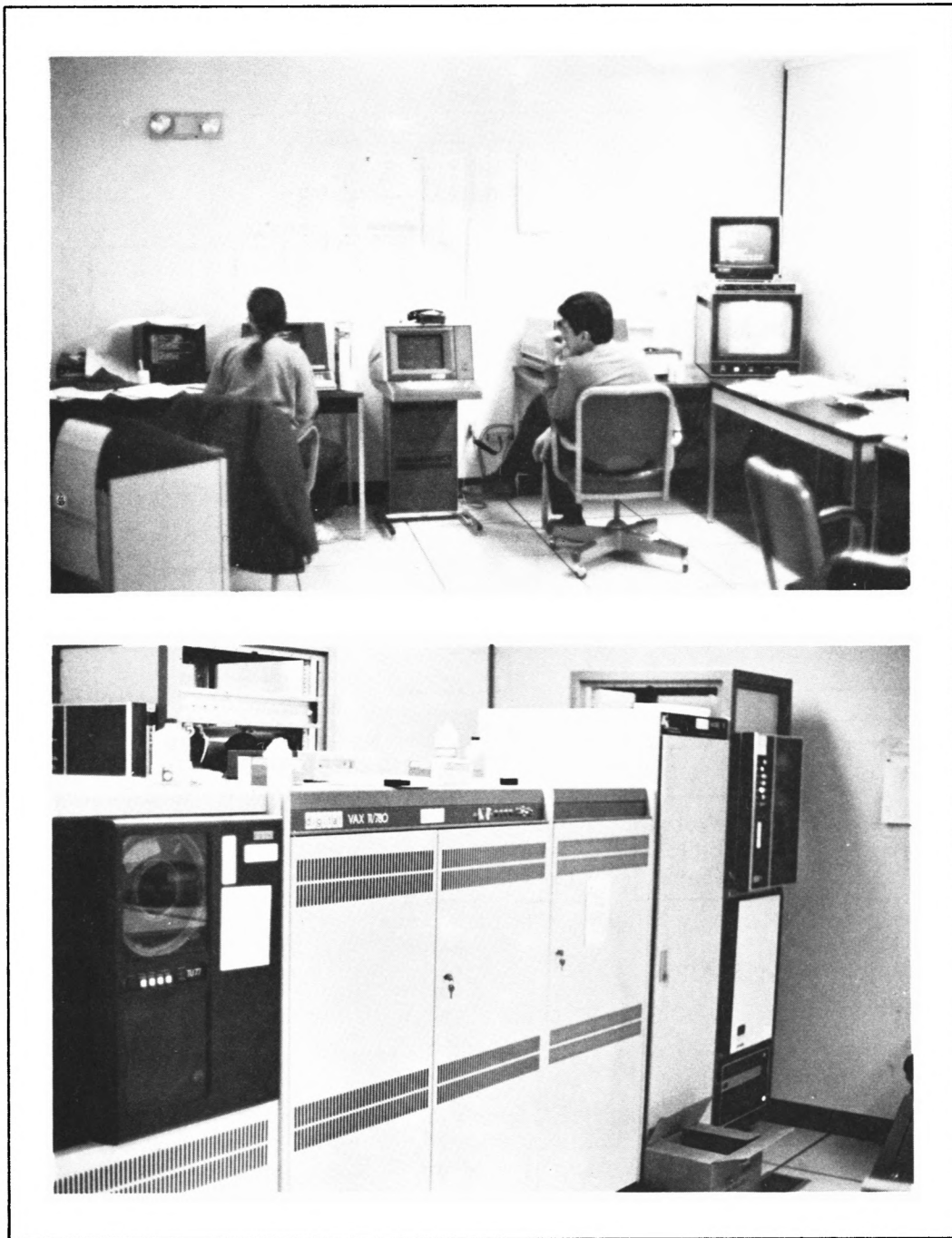
Figure 11-1. The top photographs shows two users running AIPS on a single VAX. Both are running AIPS on TEK 4025 terminals, but sharing use of the TEK 4012 graphics terminal in the center, the image display CRT at the far right, an array processor, a VERSATEC printer-plotter, and tape drives. Each user has an AIPS task-monitoring CRT; for the user at the left it is on a table to the left, while for the user at the right it is on top of the I 2 S 512 2 image display screen.
