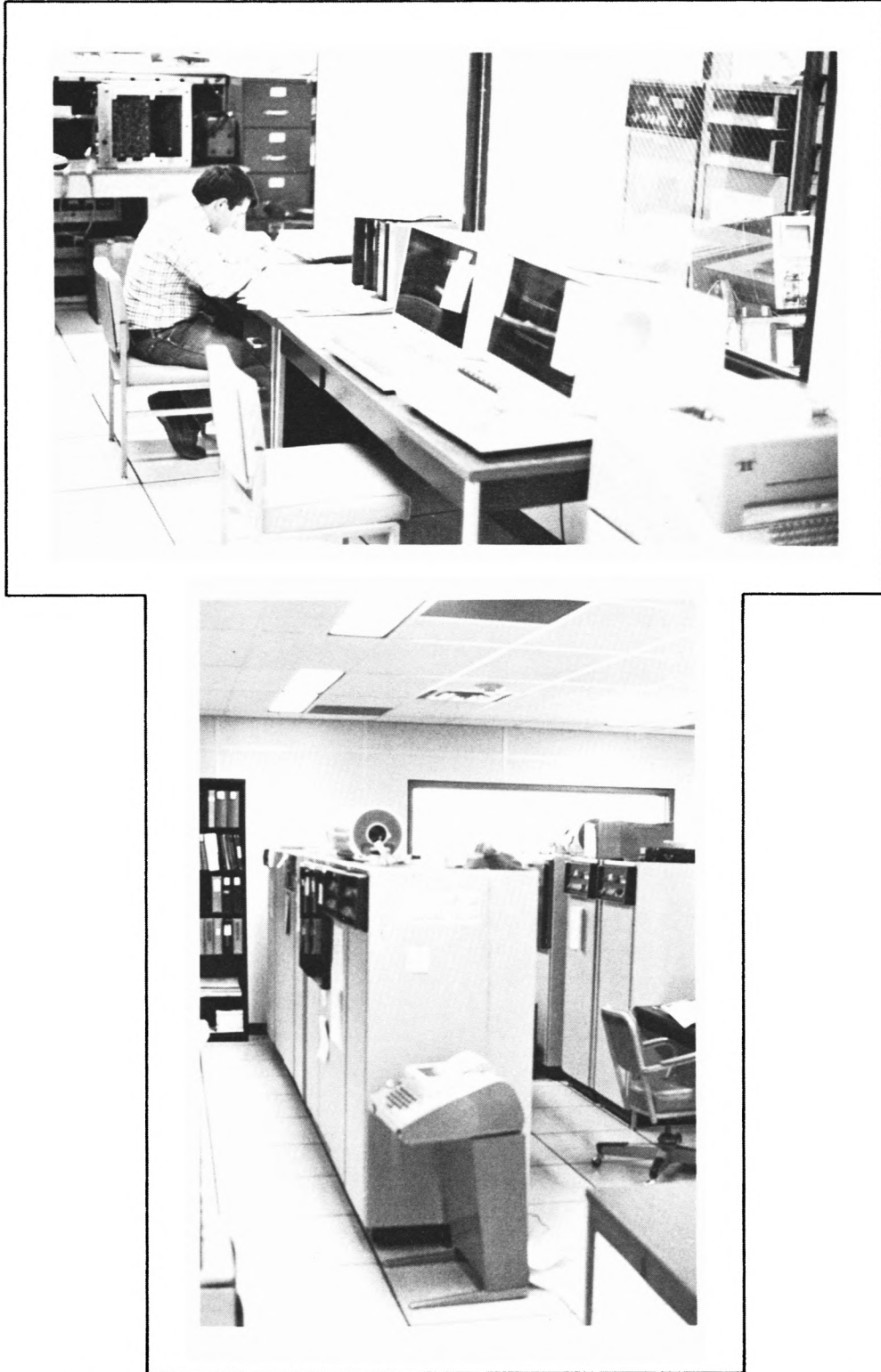
Figure 4-2. Two photographs of the MODCOMP minicomputers of the on-line computer system. The top picture shows SPECTRE and some communications terminals. The bottom picture shows the remaining on-line MODCOMP minicomputers in the main computer room.
