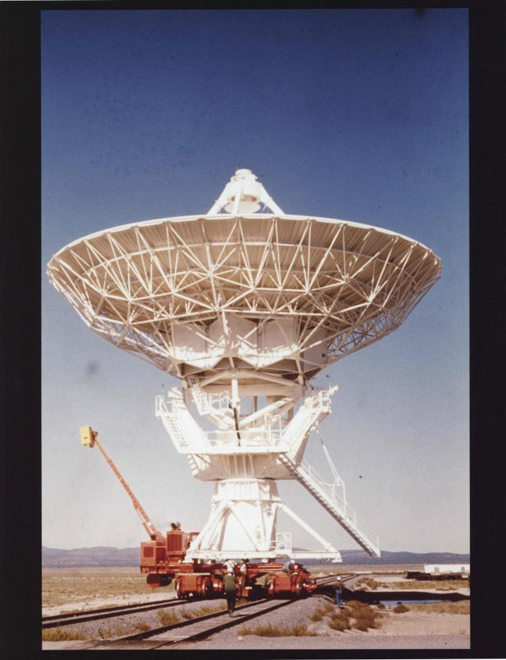
VLA Photo No. 3. Ground view of a 235-ton antenna on its 80-ton transporter moving along the double track railway. The reflector has an accuracy of 0.5 mm or 0.020 inches, rms. The movable reflector weighs in excess of 100-tons.
