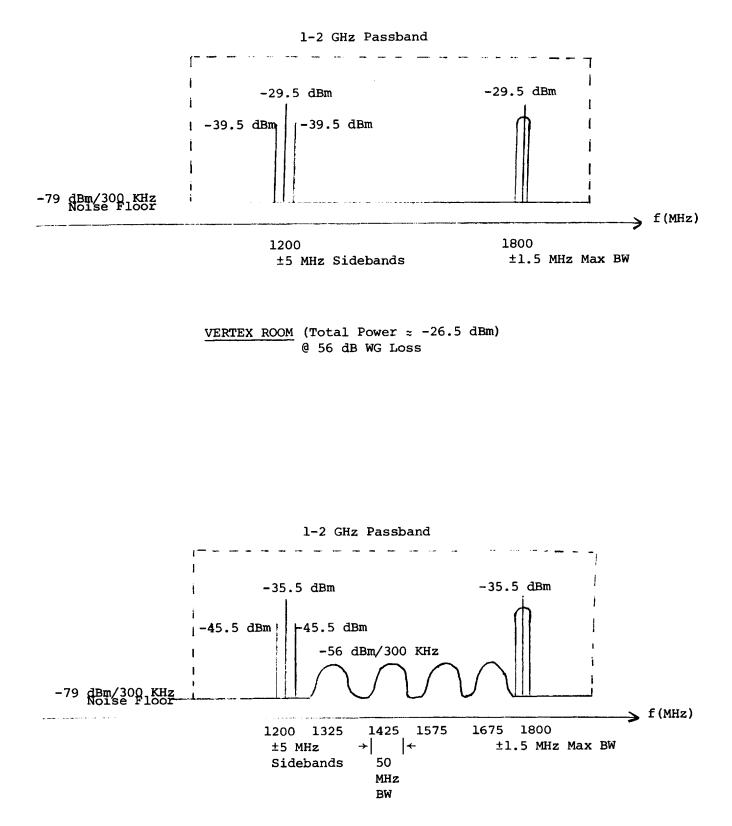
CONTROL ROOM (Total Power  $\approx$  -26.5 dBm) @ 56 dB WG Loss
