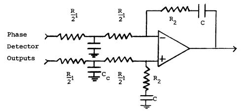
The time constant of this network as recommended by the Motorola MC4044 (similar to the MC12040) data sheet (p.9) should be given as below.
