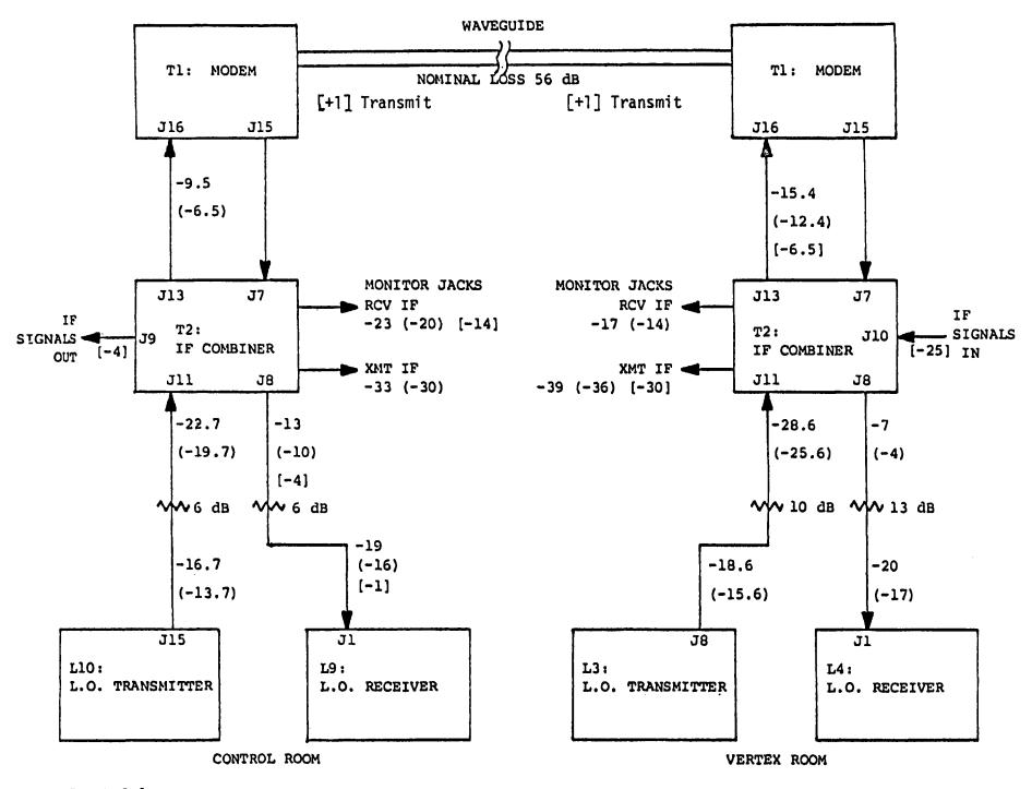
FIGURE 3-1: System levels and pads. All power levels in dBm and apply to carrier if no parenthesis, total LO carriers if in parenthesis, and total IF and LO power if in brackets. All signal levels are when the signal is ON; they are not average levels.
