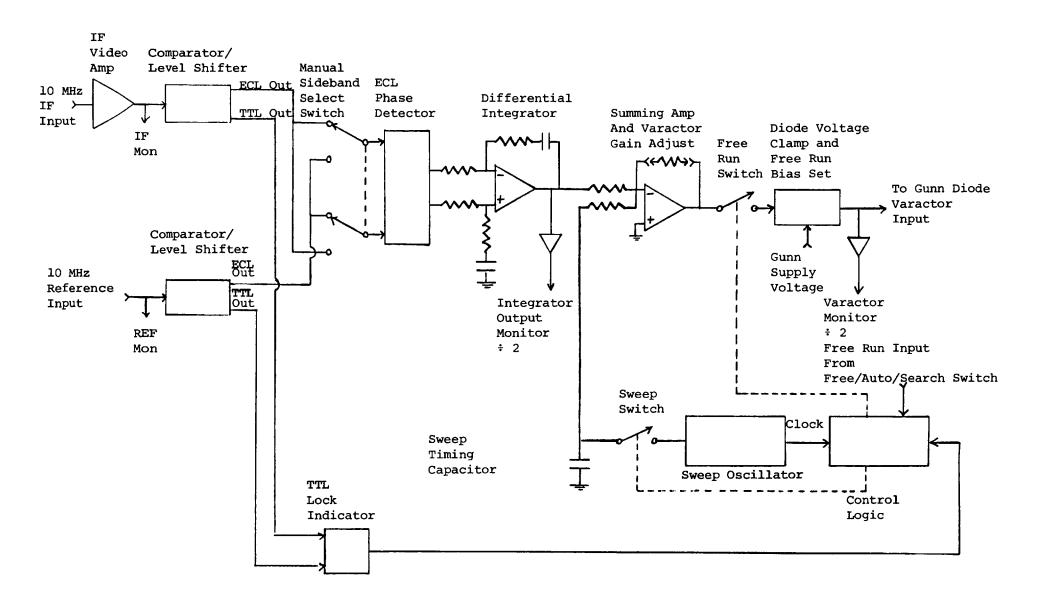
FIGURE 4-5: PHASE LOCK UNIT BLOCK DIAGRAM
