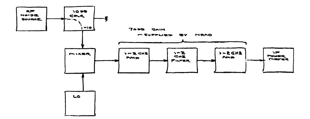
FIGURE 3 - Noise figure measurement set-up.
