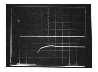
TOP TRACE - T/R Input Pulse (Vertical 2 Volts/Div) (Horizontal 0.5 µS/Div)
