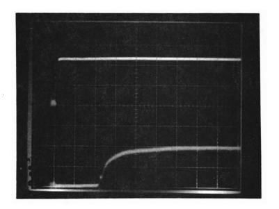
TOP TRACE - T/R Pulse (Vertical l Volt/Div) (Horizontal 0.5 µS/Div) BOTTOM TRACE - Detected Receive Output At T2-J8 (Vertical 50mV/Div) (Horizontal 0.5 µS/Div) MODULES USED - T1D14 (phase locked) and T2B5
