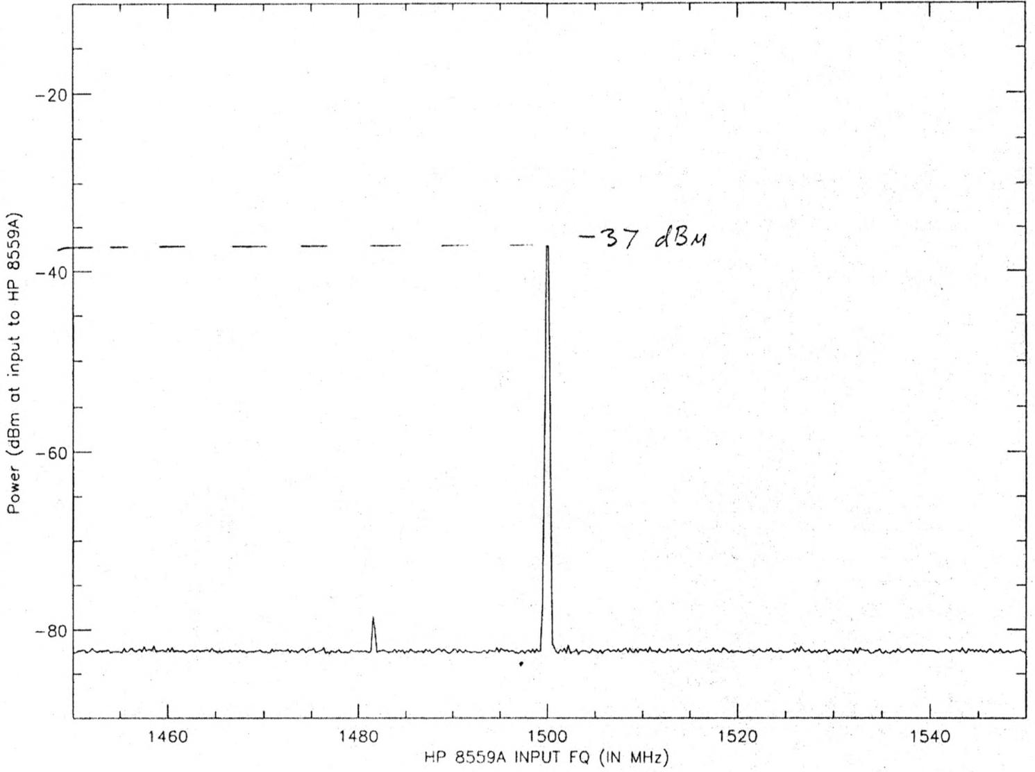
Note: Signal detected at 1481 MHz is a miscellaneous signal; not a part of the experiment
