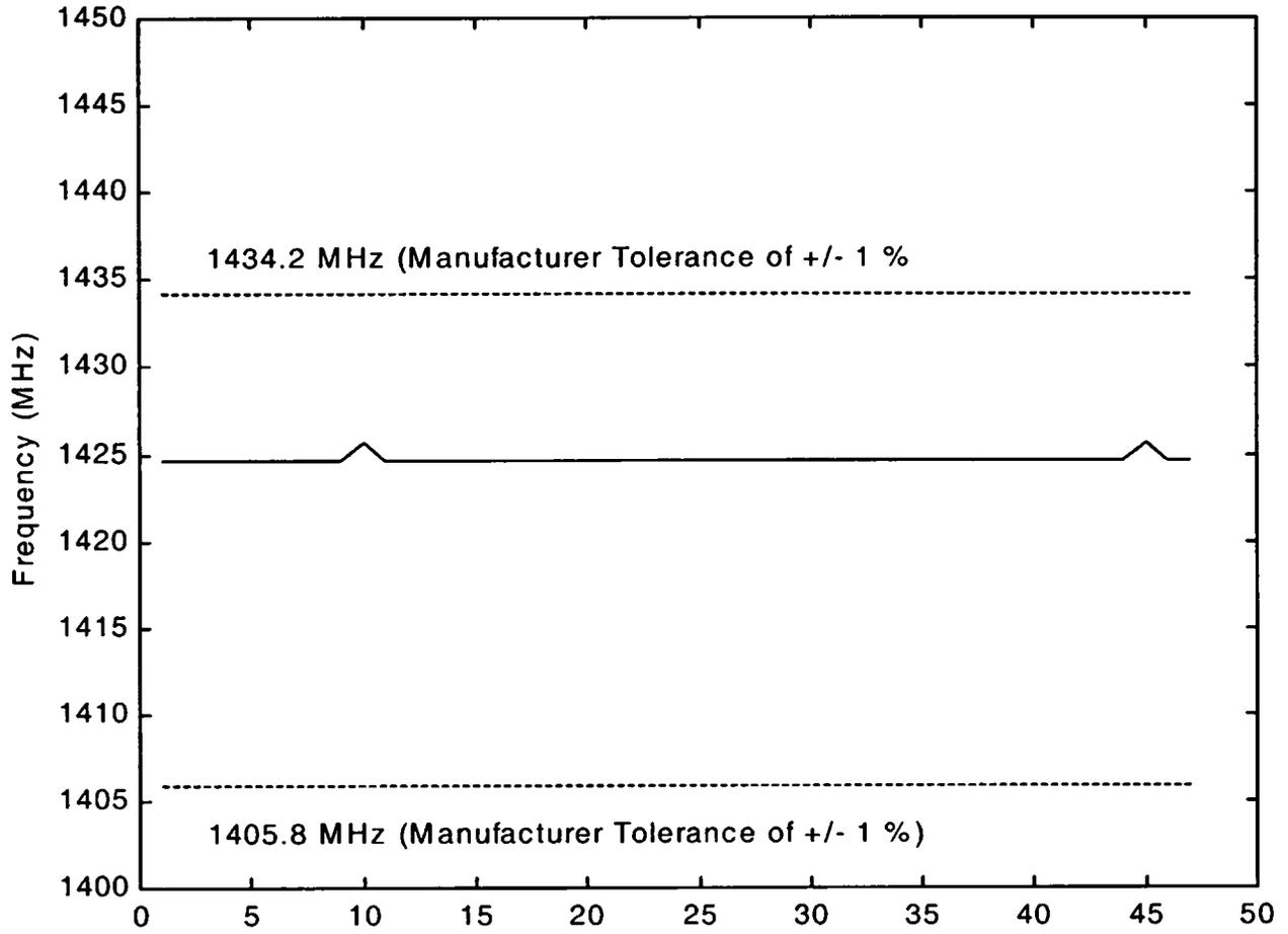
Scan # (1-47): Solid Line is Rx Performance; Dashed Line indicates Manufacturer Tolerances
