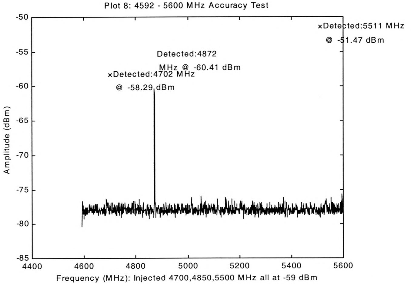
Plot 8.1a: Repeatability Test for a 4850 MHz Injection at -59 dBm; 4592 - 5600 MHz Scan)
