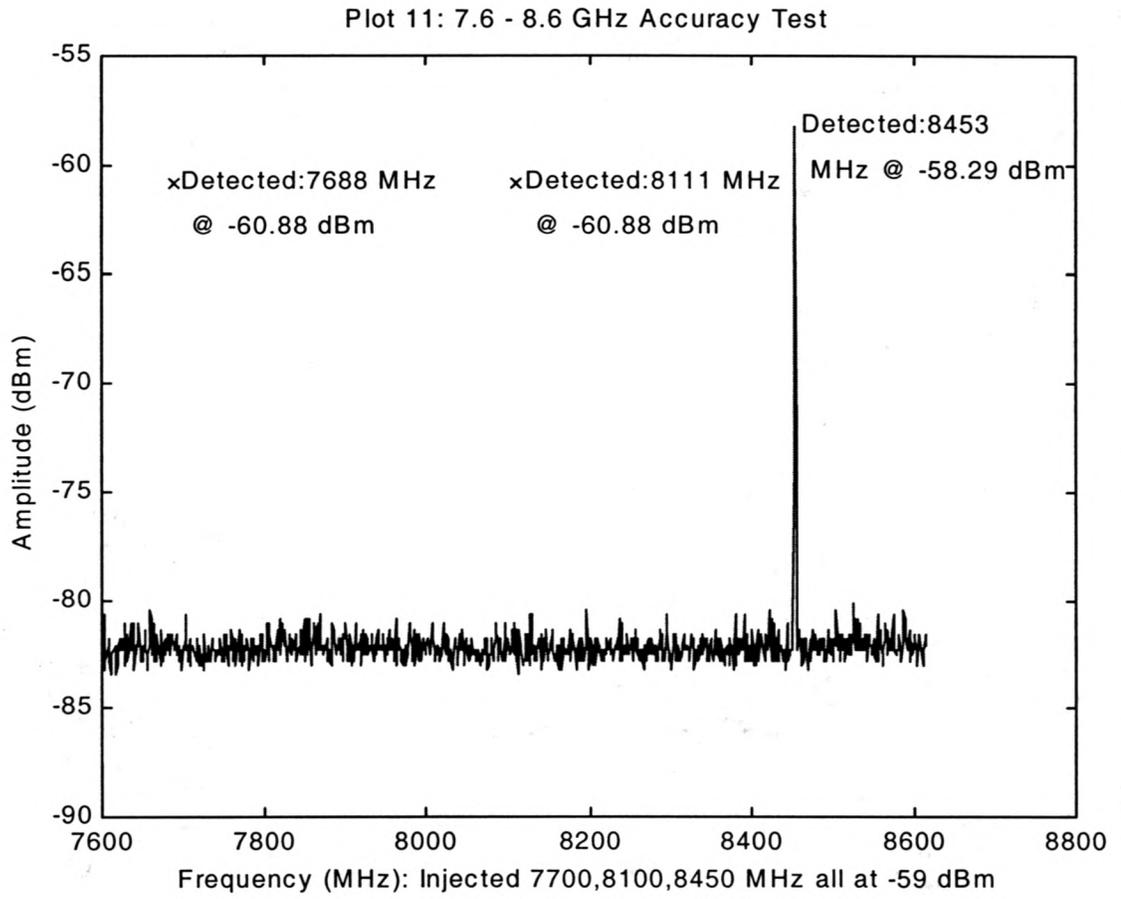
Plot 11.1a: Repeatability Test for a 8450 MHz Injection at -59 dBm; 7600 - 8615 MHz Scan)
