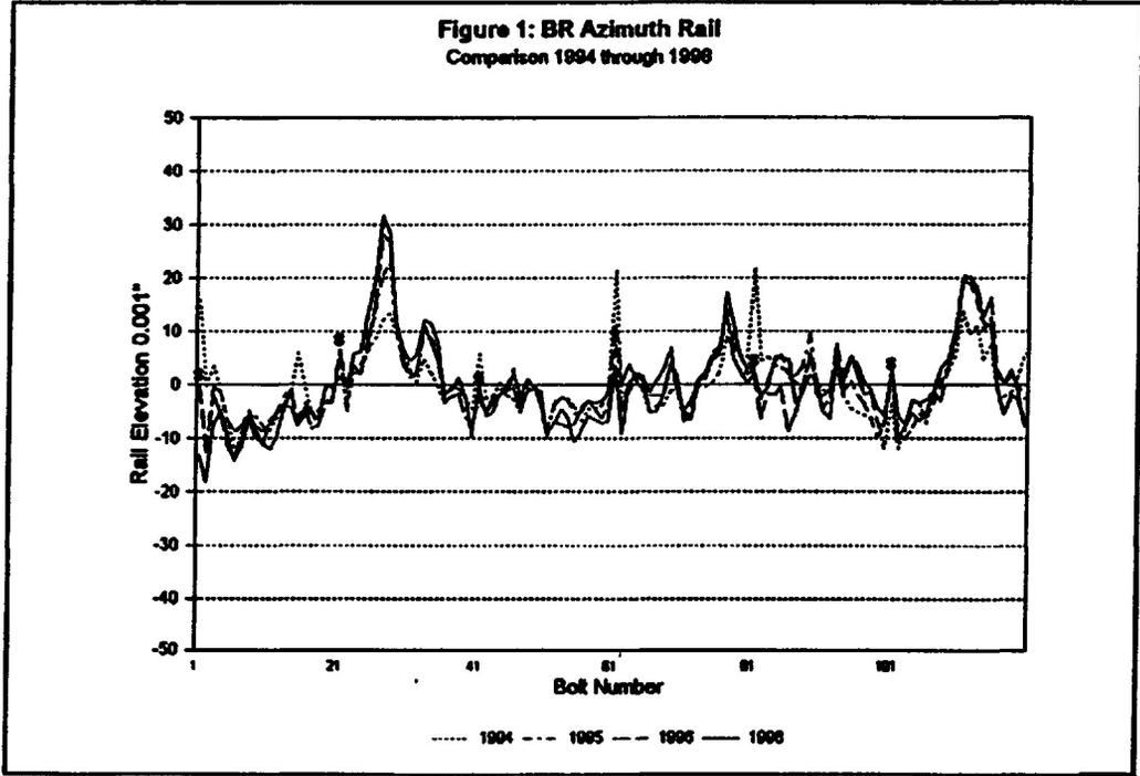
This rail and supporting grout seems to be much more stable than the rails we have been repairing. There has been little movement since 1996. There is an
