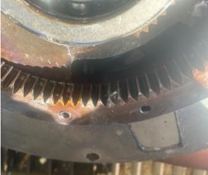
Figure 11: EL #2 Damaged Ring Gear
