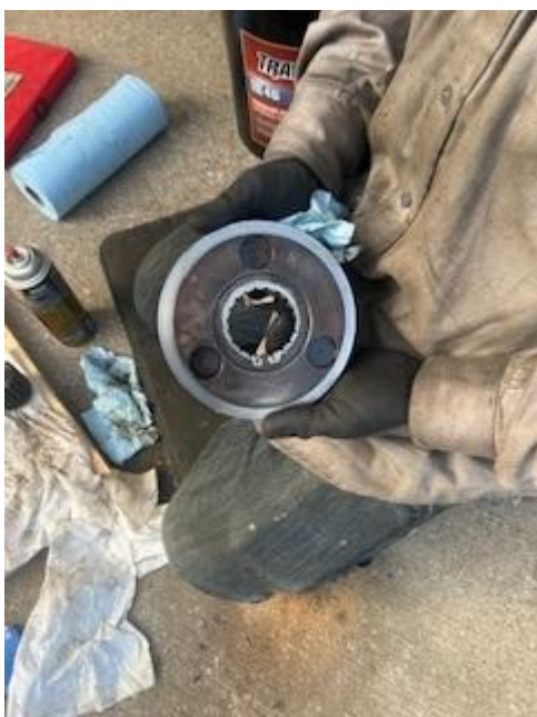
Figure 15: First Stage Carrier (Rear View)
