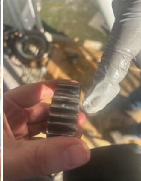
Figure 12: EL #2 Damaged Planetary Gear
