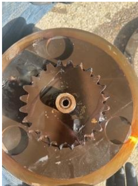
Figure 18: 4th Stage Sun (Rear View)
