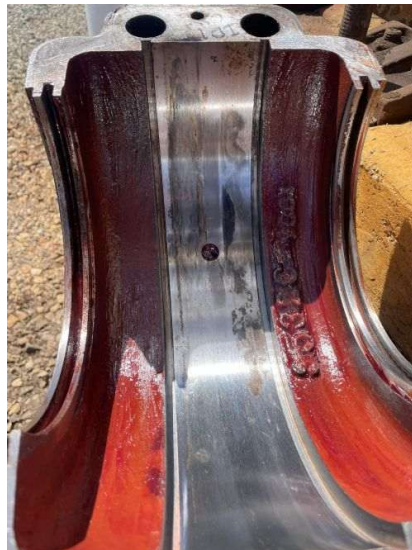
Figure 15: AZ1 idler wheel split pillow block
