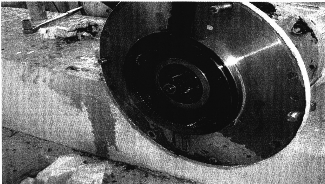
Azimuth #2 gearbox pre-load inspection. Both gearboxes showed very little signs of wear. Both gearboxes oil was changed and several flow gauges were replaced. A gearbox oil seal was replaced on AZ #1.
