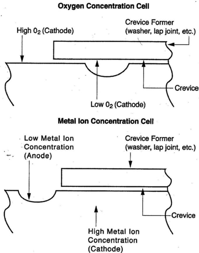
**FIGURE 1** Concentration cell corrosion. Top: Oxygen concentration cell. Bottom: Metal ion concentration cell. Courtesy of SSPC: The Society for Protective Coatings; 4th Edition, *Good Painting Practice, SSPC Painting Manual, Volume I*.
