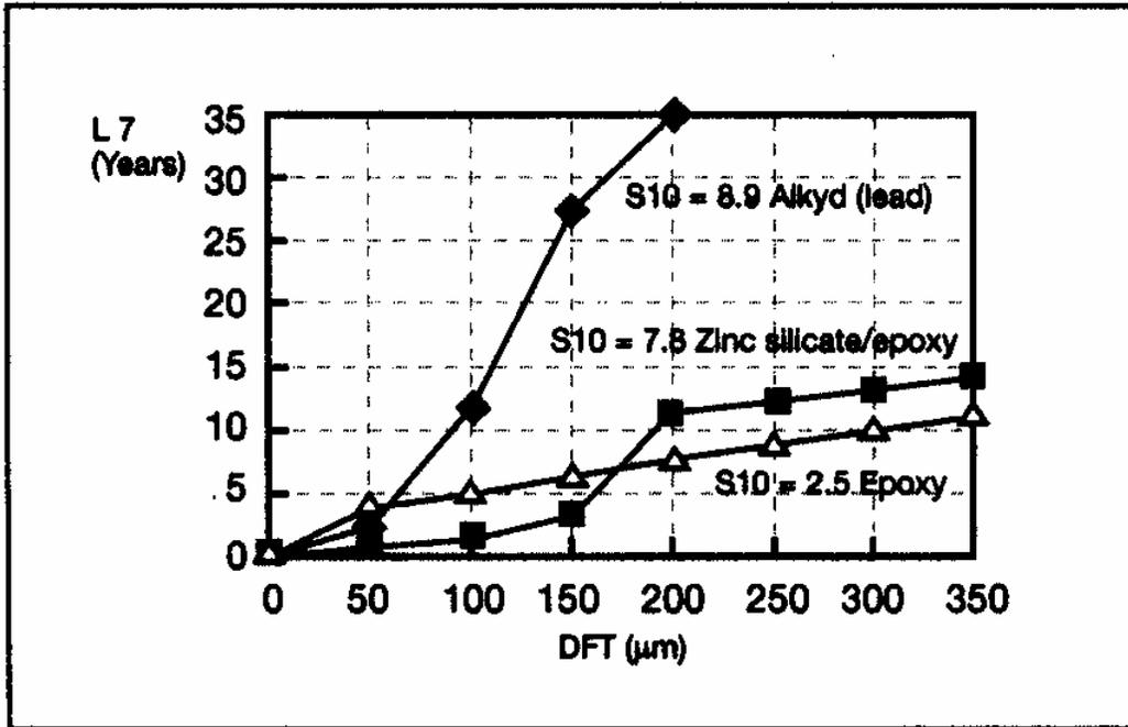
The above graph compares the time to reach rust grade 7 for 3 coating systems in a seacoast environment [24]. The St. Croix antennas Zinc Silicate/Epoxy system was specified to have a Dry Film Thickness (DFT) of 275-375 µm. According to the chart, this represents an L7 life of 13 – 14 years. The antenna was built in 1992 and is now 15 years old.
