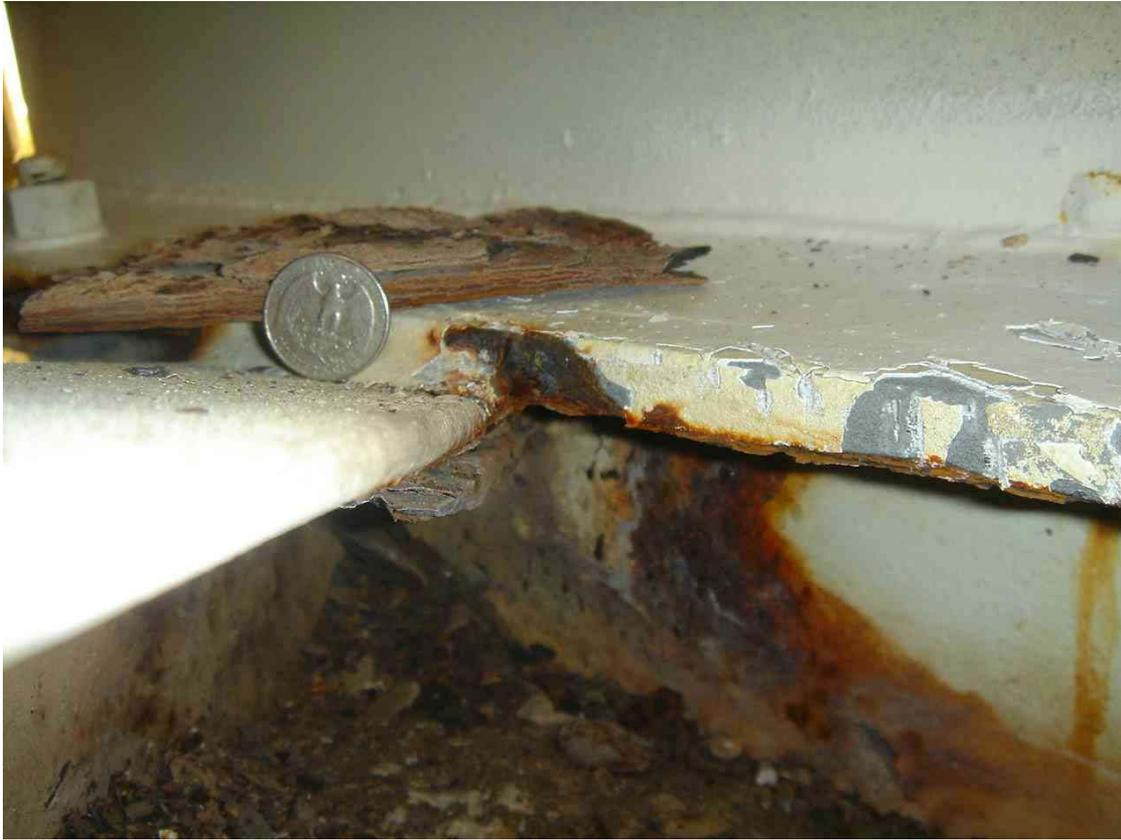
The steel is beginning to swell and disintegrate and flakes off in layers. This form of corrosion is called exfoliation. Exfoliation is a form of layer corrosion which starts at the edge, proceeds within the body of the material in paths parallel to the rolling direction of the steel. The corrosion formed is greater in volume than the metal it replaced, and the layers of steel are forced apart.
