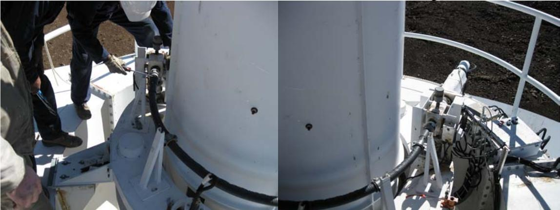
The FRM was given thorough inspection and the focus flex shaft was replaced.
