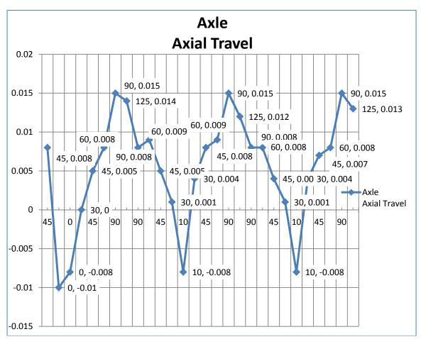
The graph shows that there is a maximum of .007" of hysteresis occurring at 90 degrees, but that the repeatability when moving the axis in the same direction seems to be better with a maximum difference of about .004" at 30 degrees travelling up.
