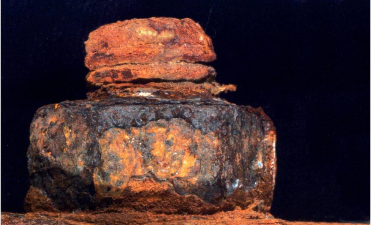
Figure 4: failed PTFE/nickel plated low-alloy nut and bolt after 18 months in splash zone
