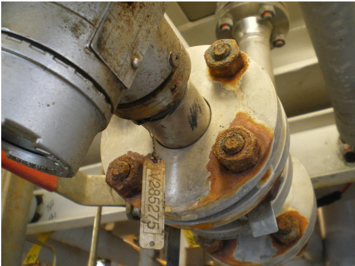
Figure 3: salt spray affected low-alloy bolts in high-alloy substrate
