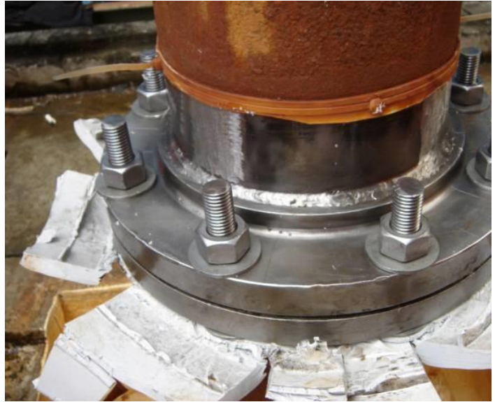
Figures 18 & 19: bare steel substrate show no sign of corrosion after 6 months
