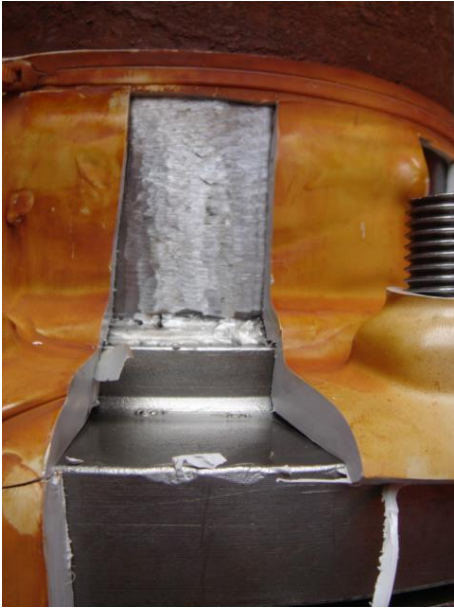
Figures 18 & 19: bare steel substrate show no sign of corrosion after 6 months
