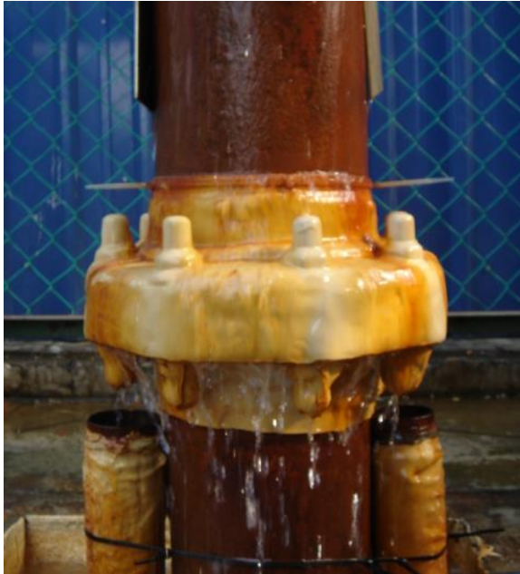
Figures 16 & 17: Pipe at beginning of salt water deluge testing and after 2 months
