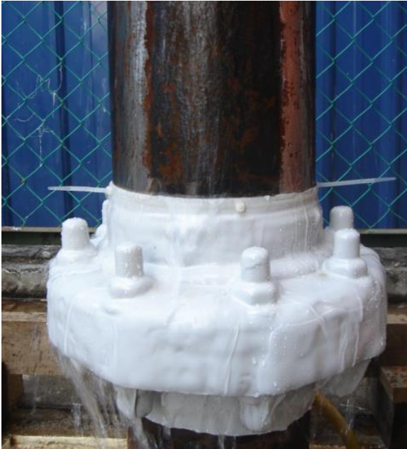
Figures 16 & 17: Pipe at beginning of salt water deluge testing and after 2 months
