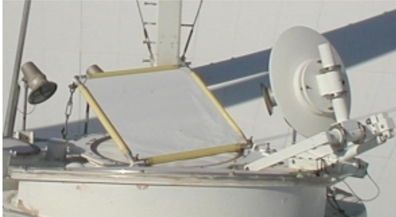
**Figure 1: Dichroic Reflector**
