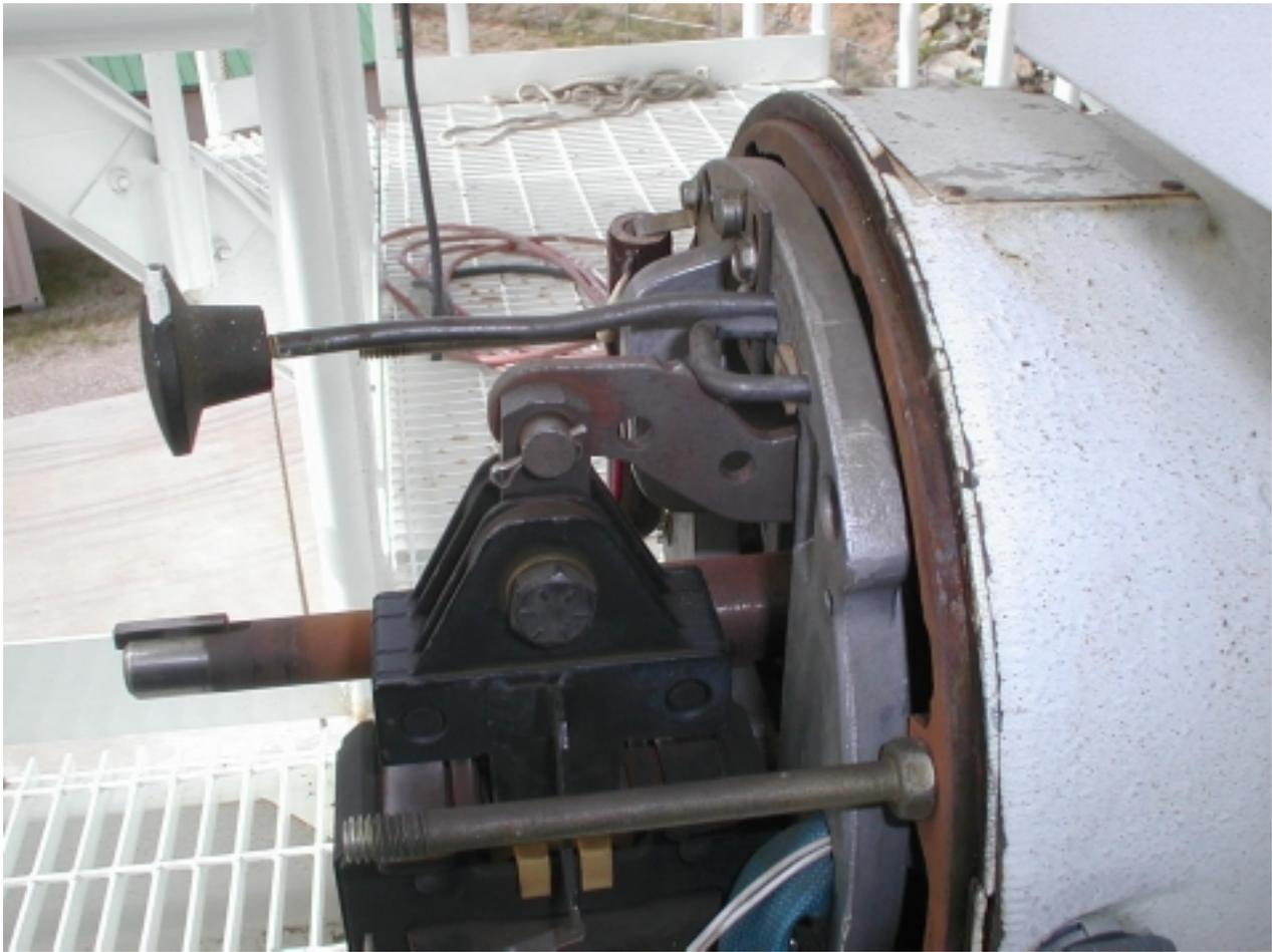
Figure 14: Brake lever stuck in mid travel
