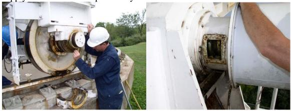
Azimuth wheel bearings were inspected. Site Techs should remove excess grease from the elevation encoder bearing more frequently.
