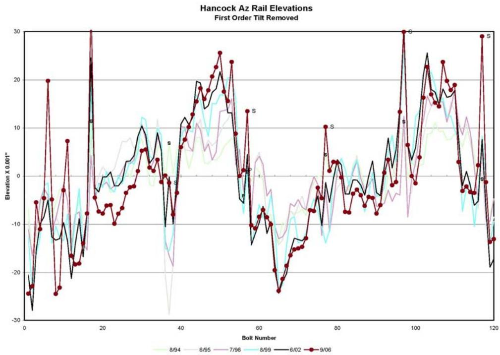
Splices at bolt numbers, 17, 97 and 117 are failing.
