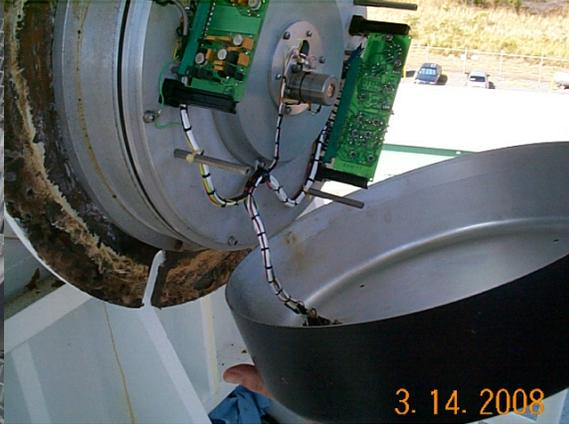
Elevation motor #2 was replaced. Grease was found inside the elevation encoder during the inspection and will have to be replaced.
