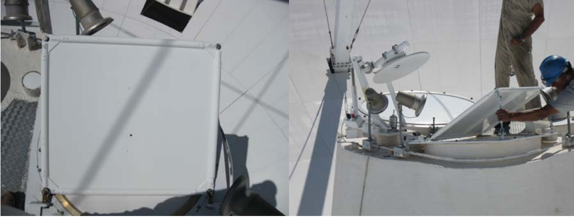
The old Dichroic reflector was delaminating and could not be aligned. The reflector was replaced and the new one aligned.
