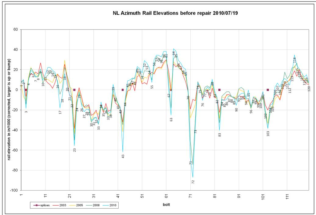
Figure 1: Rail height since last repair
