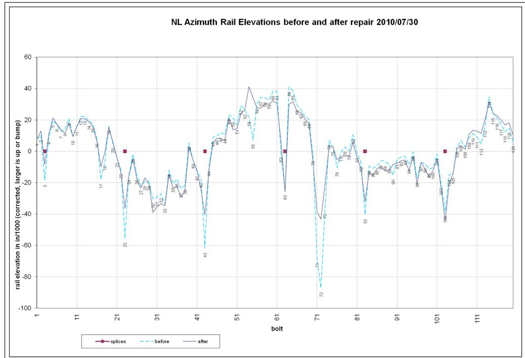
Figure 13: Rail height before and after repair
