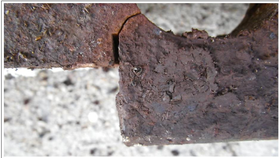
Figure 9: Splice bar typical cracks at North Liberty antenna
