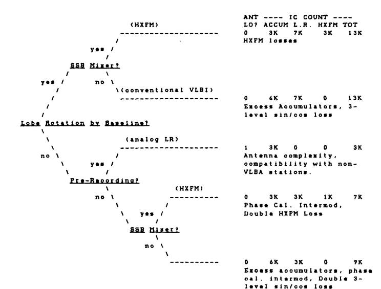
HXFM = Digital (discrete) Hilbert Transform SSB Mixer = Digital SSB mixer using HXFM
