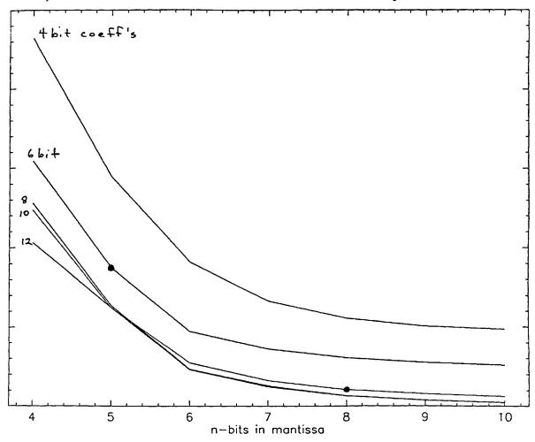
FX-style FFT vs. conventional FFT. Errors in monochromatic signals.
