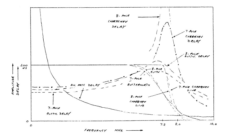
FIGURE 2 BANDPASS + DELAYS
