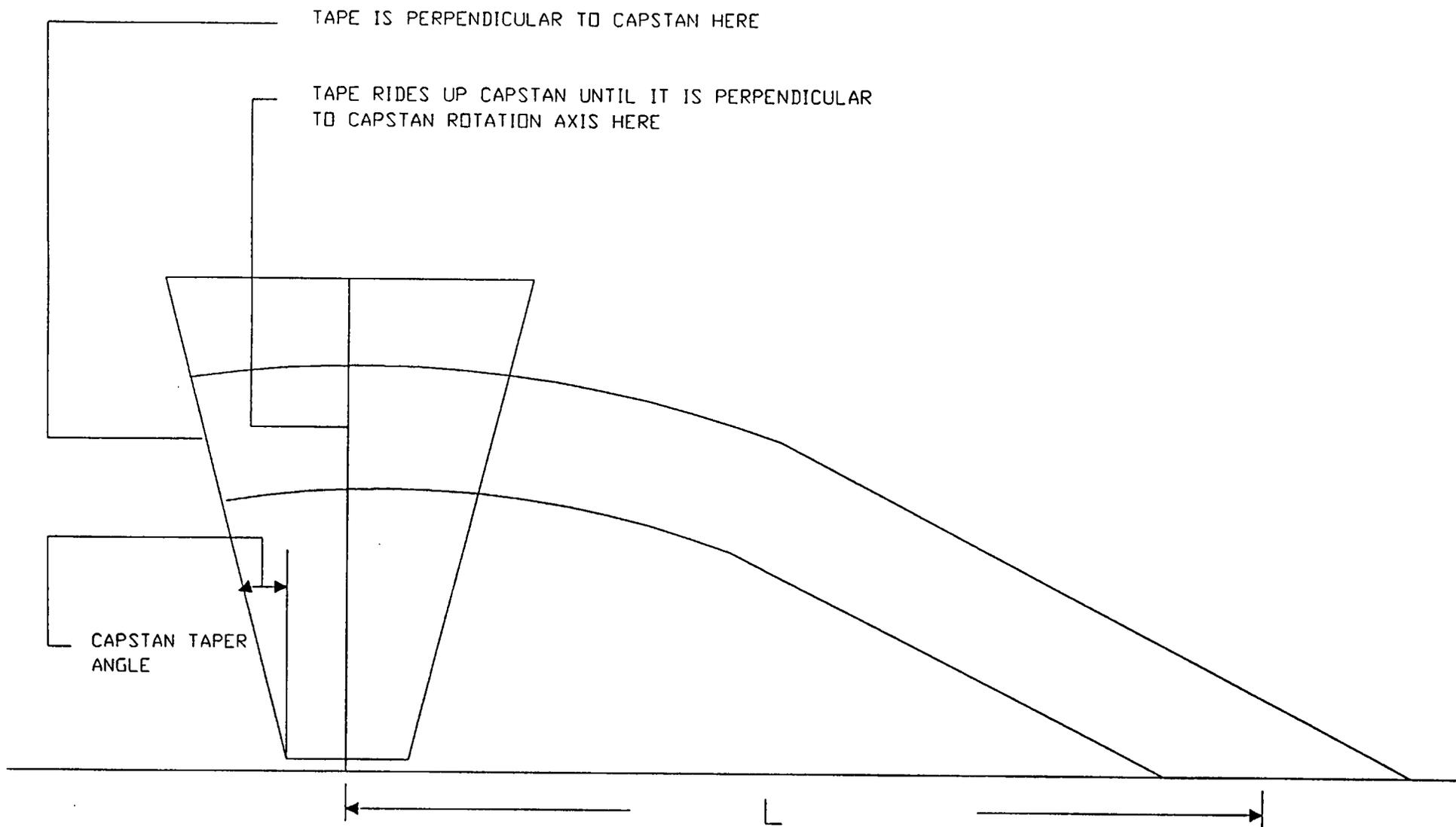
FIG 1 BENDING BEAM MODEL OF TAPE PATH UNDER ACTION OF A CAPSTAN WITH TAPER
